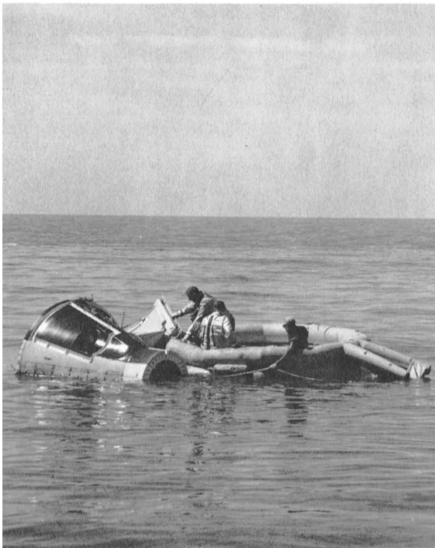
WATER EGRESS procedures are developed through testing procedures. Two astronauts are shown here after practicing egress from a boilerplate Gemini spacecraft in Galveston Bay.
