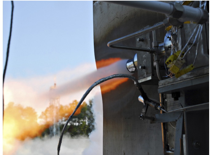
Engineers at the Marshall Center conduct a battery of tests on the J-2X’s workhorse gas generator, the driver for the turbopumps which start the engine for the Ares I rocket upper stage.
