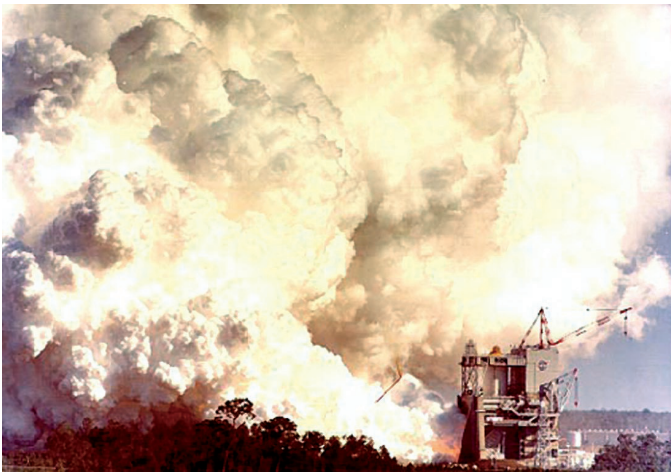
Test firing of a Saturn V second stage rocket in April 1966. The rocket used a cluster of five J-2 engines. (NASA/SSC)
