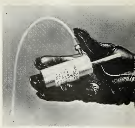
THIS Arthur D. Little-developed min-IR cooler is a low-pressure, closed-cycle refrigeration device developed for use with IR detection equipment.
