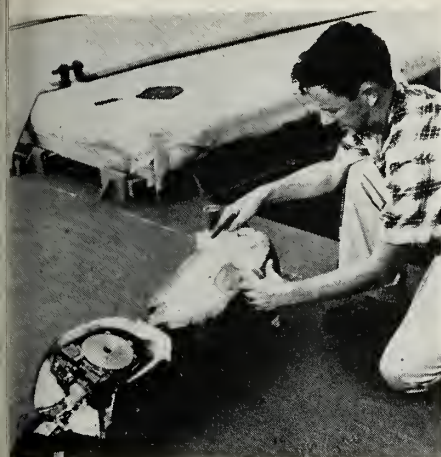
← AMPEX MR-100 tape survived Thor flight and nine days ex- posure in Atlantic.
