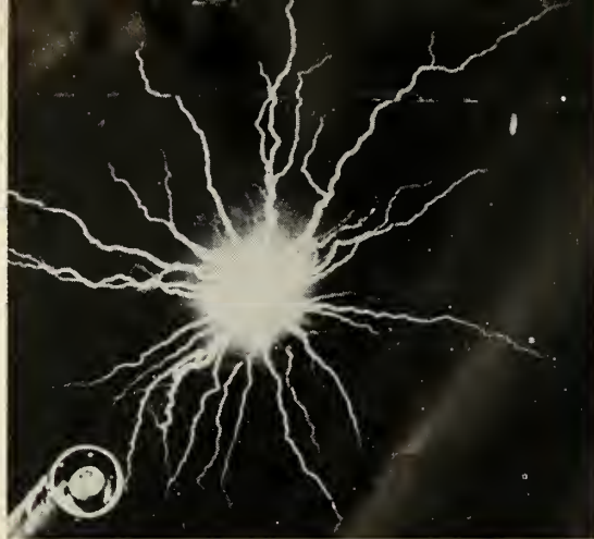
BALL OF FIRE under water. Soviet photograph of high-voltage discharge produced at Leningrad Polytechnic Institute shows that end of "projector" is coaxial cable or waveguide, seemingly corroborating idea that lightning ball is combination of electric and electromagnetic activity. Engineer Lev Alexandrovich Yutkin has charge of work.
