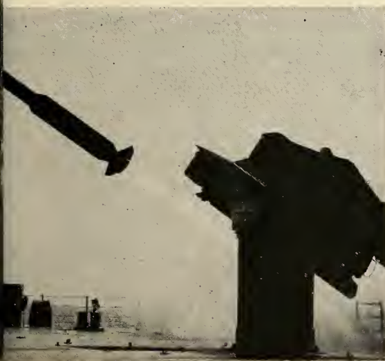
ABOARD the USS Norton Sound, a high-performance Tartar surface-to-air guided missile leaps from its launcher and streaks toward its target off the Pacific Coast. The supersonic Convair Tartar is about 15 feet long and slightly more than a foot in diameter. This photo was made from a stationary high-speed sequence camera mounted on the Norton Sound's after-deck.
