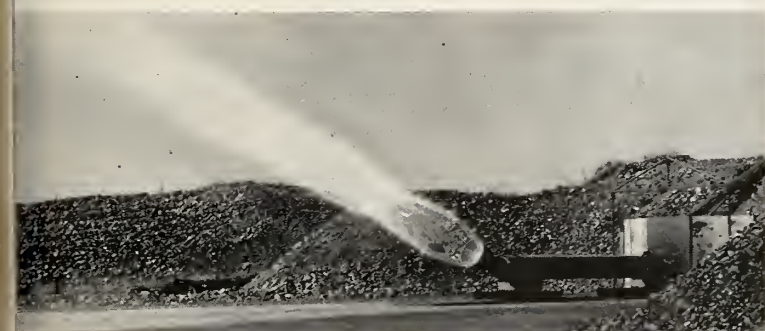
TEST FIRING by Aerojet of large solid-propellant rocket engine for guided missile launchings. The company is working on the solid propellants for the Navy's Polaris .
