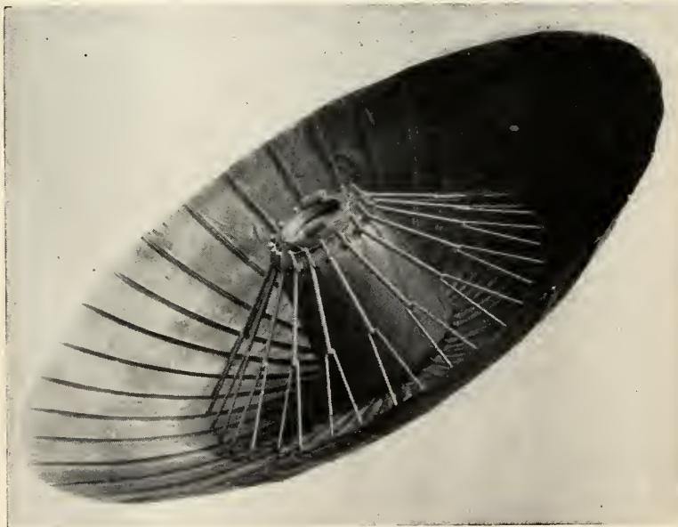
FIG. 1—Model of Avco drag brake. Mechanical engineering and structural design by All American Engineering Co. in cooperation with the Avco-Everett Research Laboratory.
