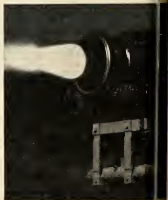
THE MEASURE OF ROCKET POWER The liquid-propellant AR engines are "static test" engines. Rocketdyne's field laboratories measure thrust and performance.
