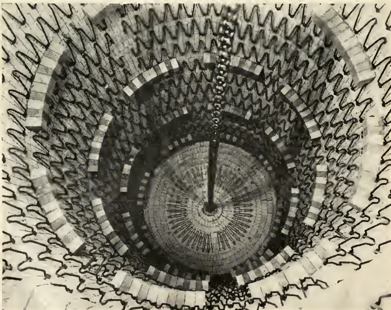
NEW CONTROLLED atmosphere hardening furnace at Lindberg Steel Treating Co.'s plant at Melrose, Ill. Furnace is big enough to take Boeing Minuteman 's rocket motor case.
