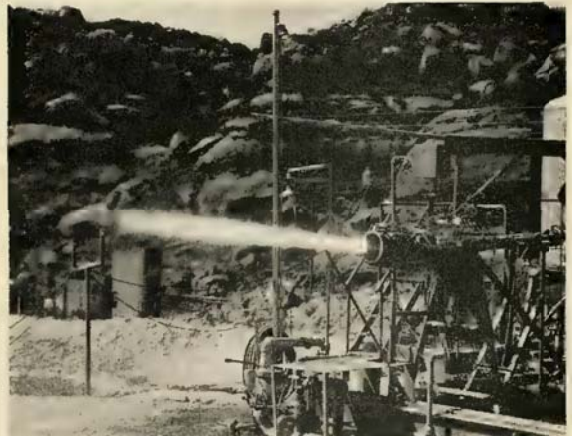
USING hydrogen peroxide and JP-series fuel, AR engines undergo static firing.
