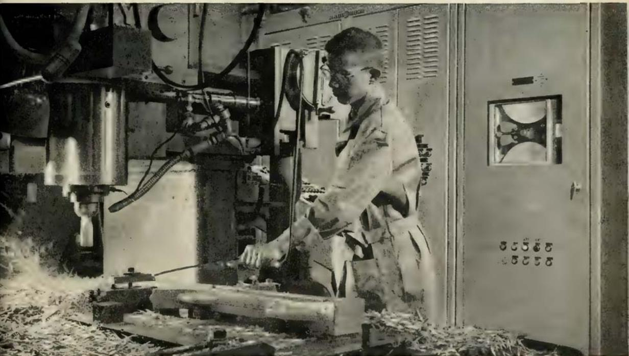
**is programmed by AMPEX tape recorders**
