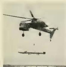
**NEW MOBILITY** for Honest John is demonstrated by the Sikorsky S-60 crane helicopter which can carry a six-ton load.
