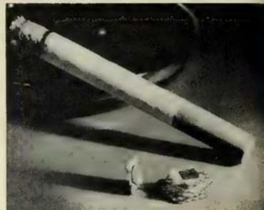
A solid tantalum capacitor half the thickness of a dime, and a tiny mercury battery the size of an aspirin have been developed for the Army Micro-Module program according to an announcement by **P. R. Mallory & Co Inc.**
