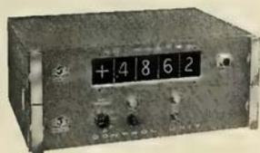
**DC MEASUREMENT:** Four and five-digit Cubic DC Voltmeters combined with the Control Unit provide instrumentation for bench-top use or for simple insertion into elaborate systems.
