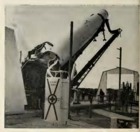
Thor IS ERECTED to vertical launch position by its transport erector on Vandenberg pad 75-1 as the protective shelter moves away.
