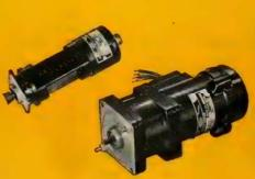
For missile applications. 2.75 HP AC motor, 3140 rpm at gear box, continuous duty, 200 volt, 400 cycle, 3 phase. Power factor: 83%. Overall efficiency: 76%. Weight: 11.25 lbs. Meets MIL-SPEC M-7969A (ASG).
