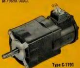
For ultracentrifuge application. 1½ HP AC motor, 12,000 rpm continuous duty, 115 volt, 60 cycle, single phase, fan cooled. Weight: 12 lbs.
