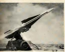
ARMY'S HAWK MISSILE is fired from mobile launcher. Missiles, launcher and support equipment can be air-lifted or quickly transported by Army or Marine ground forces.
