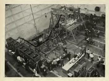
Bomarc—An Air force missile section undergoes simulated flight condition tests in Boeing Airplane Company's big new structural test laboratory. The section being tested is subjected to varying loads at elevated temperatures. Bomarc, rapidly approaching operational status, has made two remote flights from Cape Canaveral during the past month.
