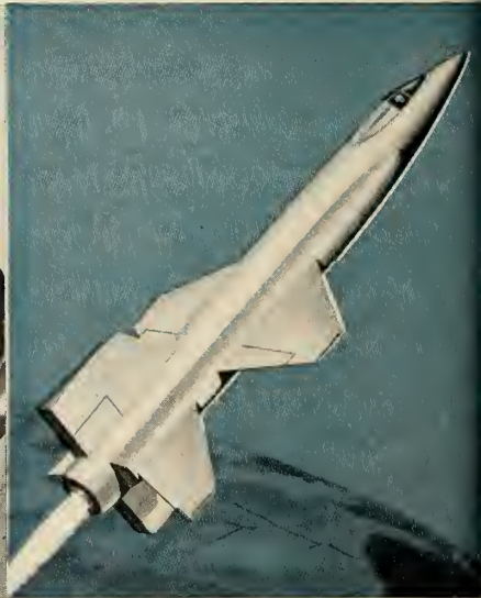
HYPERSONIC, ROCKET-POWERED X-15 manned research aircraft by North American is designed to explore near space. Sperry inertial system, developed for USAF, will give pilot data for navigating and maneuvering the NACA-sponsored X-15 with extreme accuracy at speeds of one mile per second.
