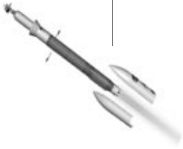
Payload fairing jettison Time: 3 minutes, 23 seconds
