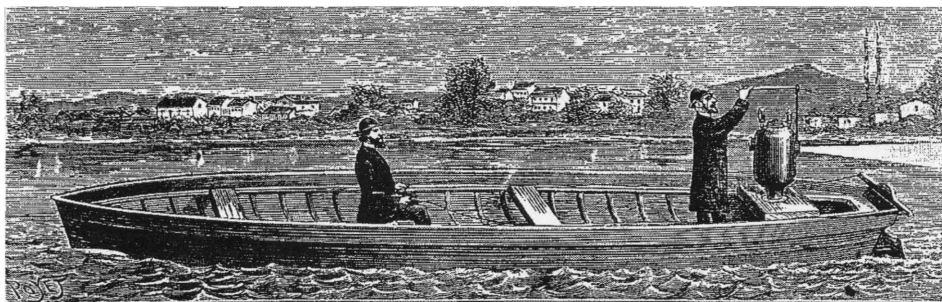
Figure 7-8: Original Model of Ciurcu’s reaction-propelled boat on Seine River, Paris, successfully tested on 3 August 1886. (From La Nature [Paris], 15 Année, 2 July 1887, p. 72).
