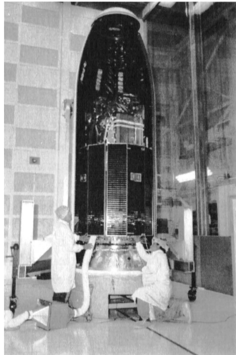
Figure 23–7: The MTI satellite, prepared for its integration with the Taurus rocket, and the Hard X-ray Spectrometer.
