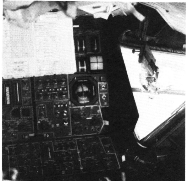
Plate 6 The Maurer DAC is shown mounted in the LM's right hand window, through which it recorded the descent to the lunar surface (AS11-36-5389).
