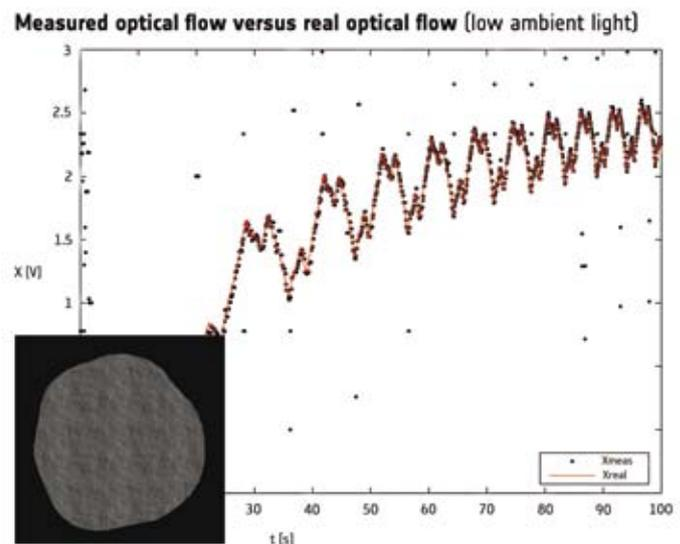
↑ Example of the performance of one of the elementary motion detectors studied (from the group at the Université de la Méditerranée in Marseille) during a fast spiral descent on a virtual asteroid (lower left corner) under critical lighting conditions as simulated using the software PANGU. Light direction is assumed for simplicity to be always at zenith. The total avionics payload of the sensor would have a mass of less than 10 g and consume less than 1W of power.
