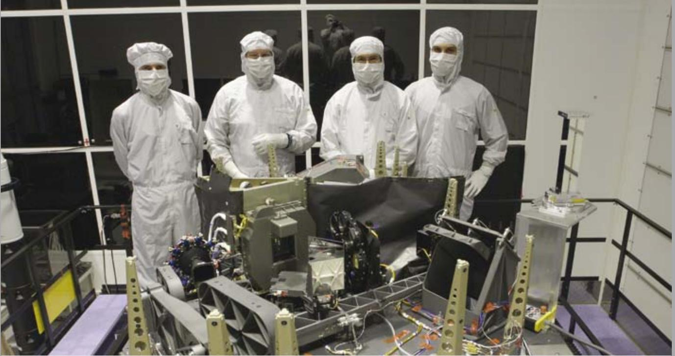
Complete integrated NIRSpec flight instrument before cover integration
