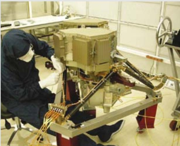
MIRI instrument ready for vibration test
