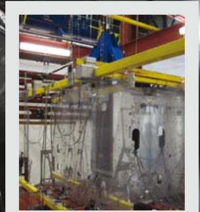
MPO Structural Thermal Model in static load test
