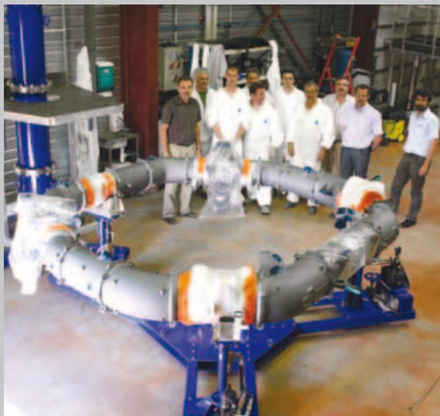
The Gaia flight model optical bench (Torus) after brazing. The hardware will undergo careful ultrasonic inspection to demonstrate suitability of the workmanship (Boostec)
