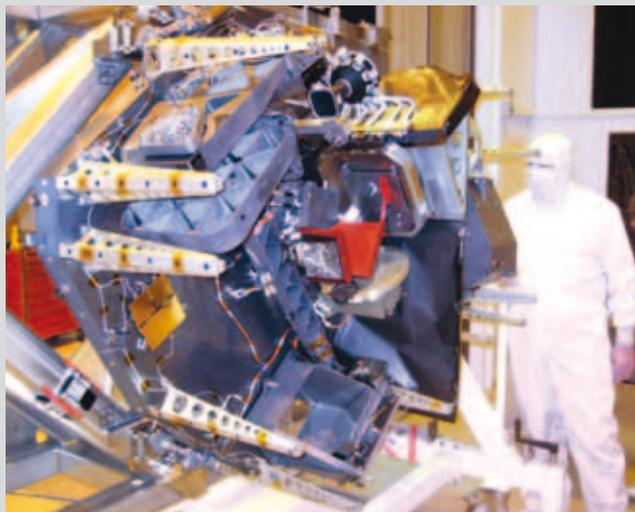
JWST NIRSpec Development Model undergoing gravity test (EADS Astrium)
