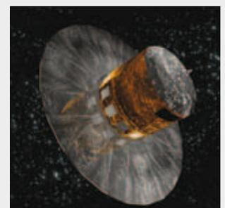
Top: Qualification Model of Gaia's sunshield during deployment testing at ESTEC, Noordwijk. Bottom left: Artist impression of Gaia's sunshield deploying; right, fully deployed
