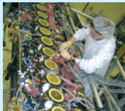
Integration of the SMOS protoflight model arm at EADS Casa Espacio
