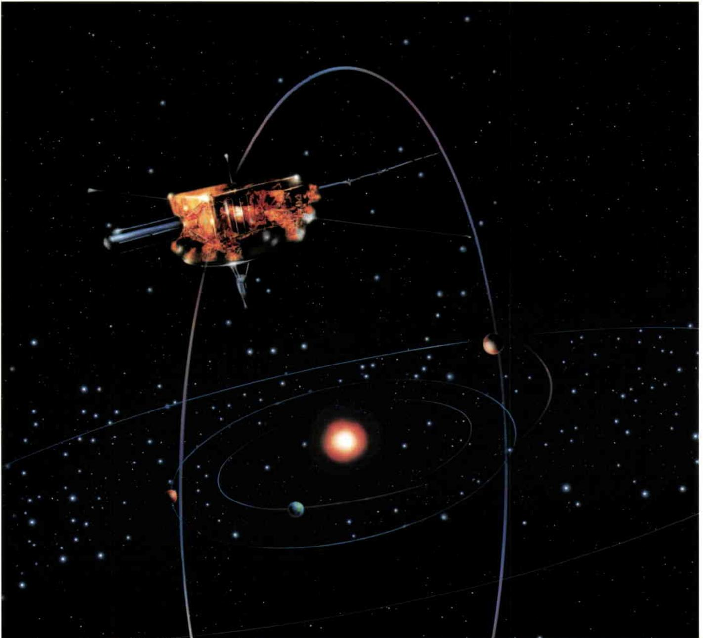
Figure 1. The first orbit of Ulysses around the Sun. The path of the spacecraft is shown in red. The red dots indicate the position of Ulysses at the beginning of each year. The Jupiter fly-by swung Ulysses out of the ecliptic (the plane in which the planets orbit) and into a solar polar orbit. Also shown are the solar passes in 1994 and 1995. The Ulysses orbit is viewed from a perspective of 15° above the ecliptic plane
