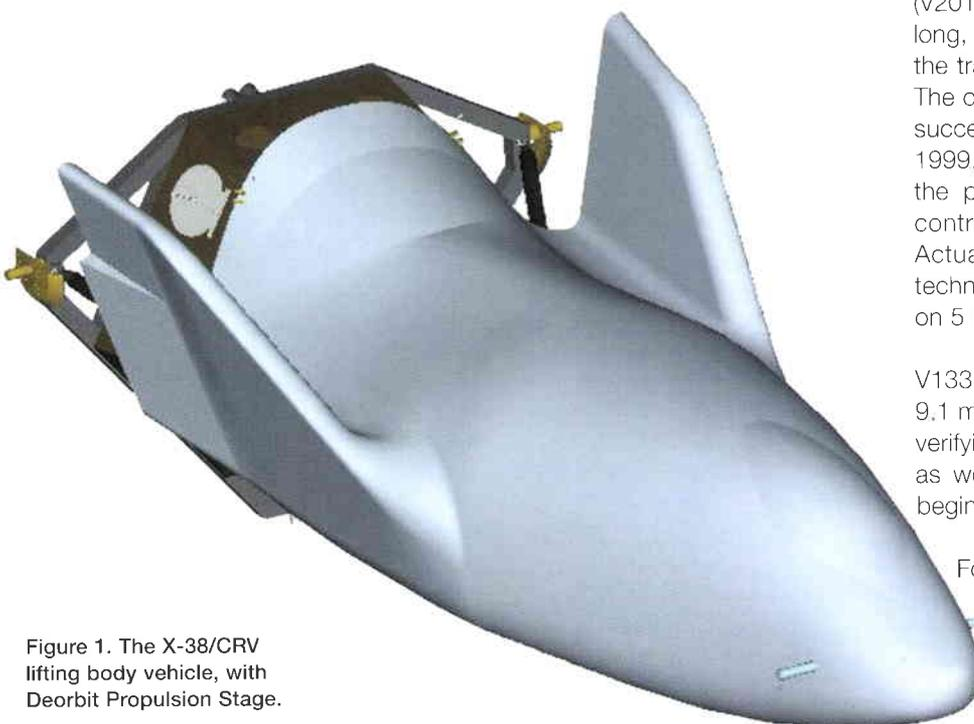
Figure 1. The X-38/CRV lifting body vehicle, with Deorbit Propulsion Stage.
