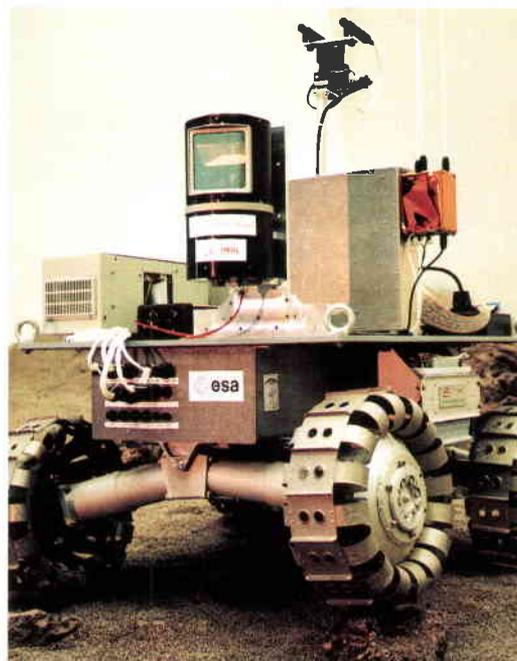
Figure 5. ASIS mounted on a rover as part of ESA's Planetary Utilisation Test-Bed
