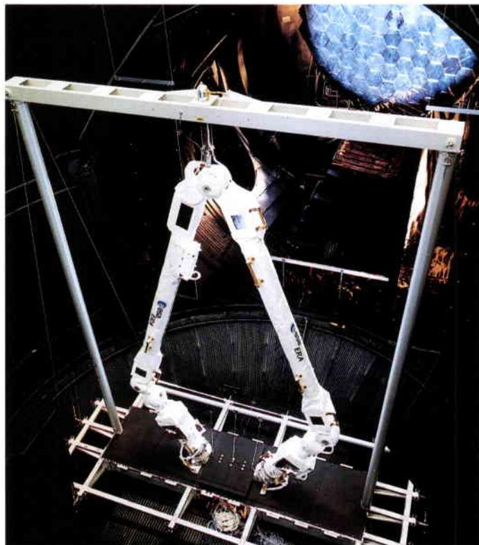
*The European Robotic Arm (ERA) in the LSS for solar simulation testing at ESTEC, Noordwijk*
