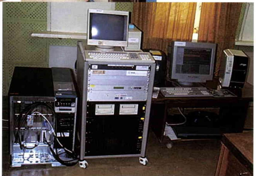
Figure 9. The ESA compact-station Multi-mission Direct Ingestion and Processing System operated by RKA in Moscow
