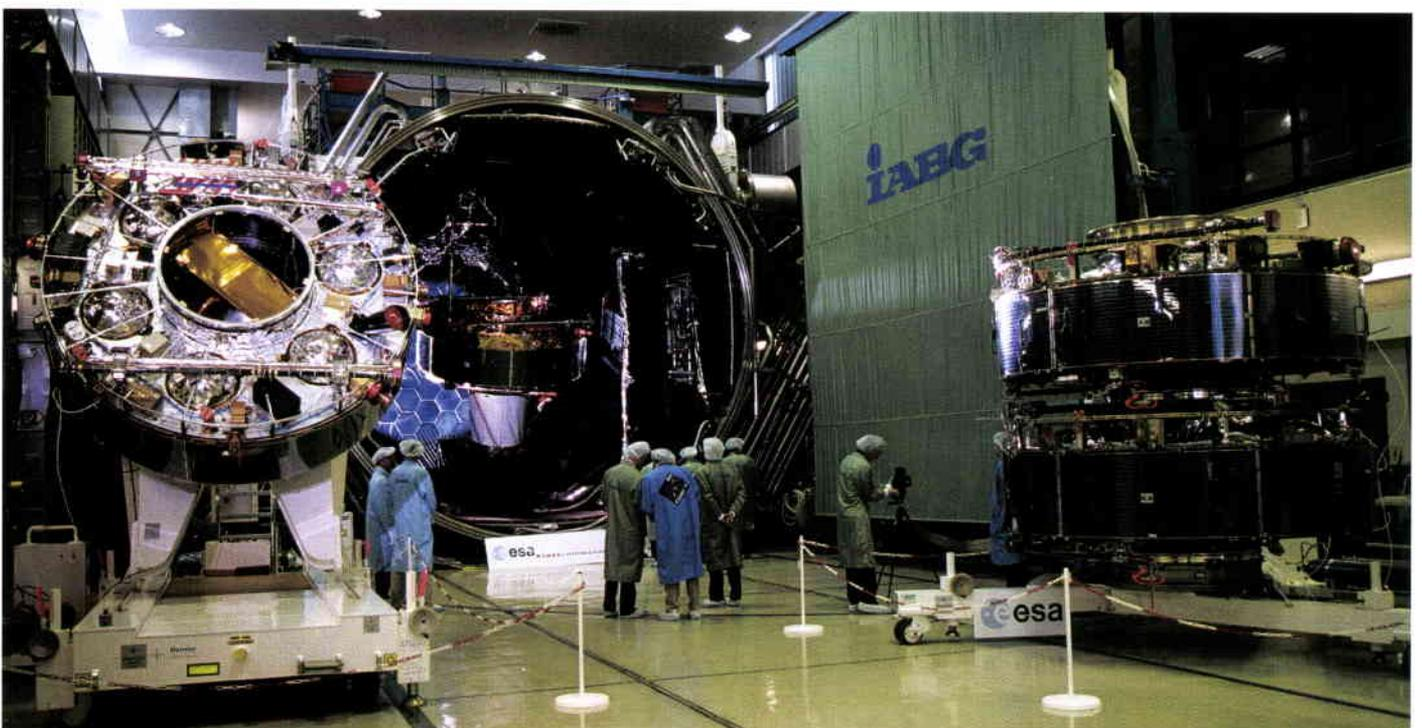
containers at IABG prior to shipment to the Baikonur launch site in Kazakhstan this spring. In the case of the other two flight models, installation of the science payloads had been completed, but their exhaustive series of environmental tests at IABG had yet to begin.
