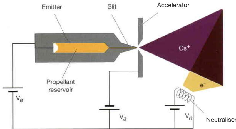
Figure 6. Working principle of a field-emission thruster
