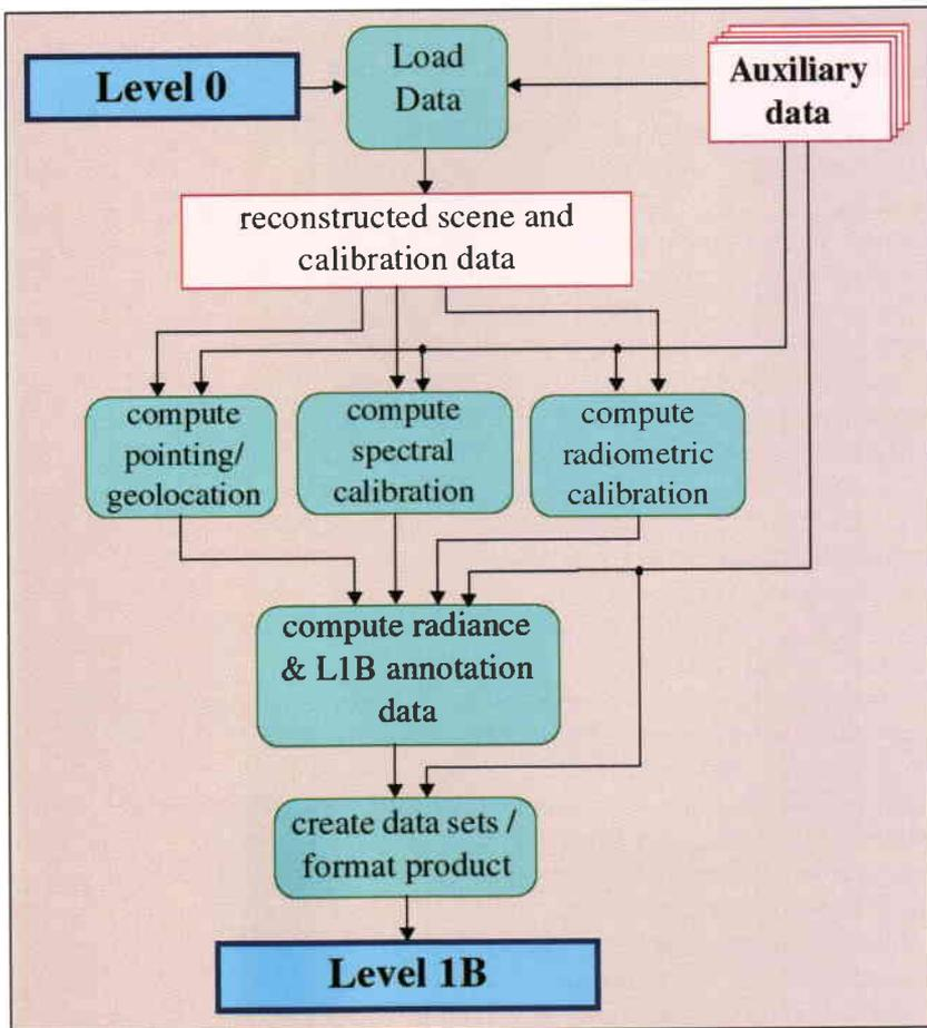
Figure 11. Level 1B processing steps
