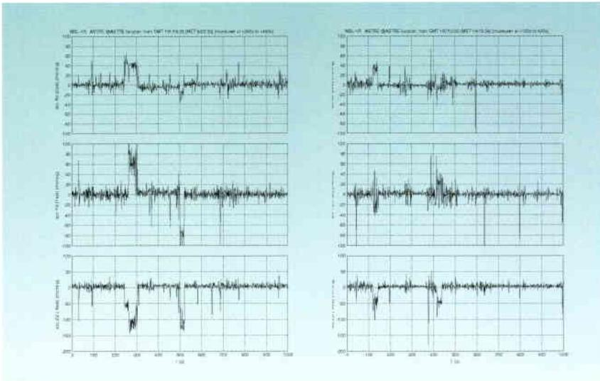
Figure 5. Evaluation of the drag modelled by the Drag Temperature Model of Barlier along each B axis from GMT 195/00. Amplitudes in mg versus time in hours
