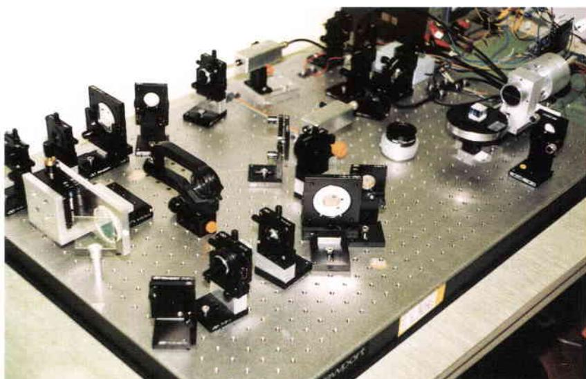
Figure 3. FMCW laser radar optical breadboard
