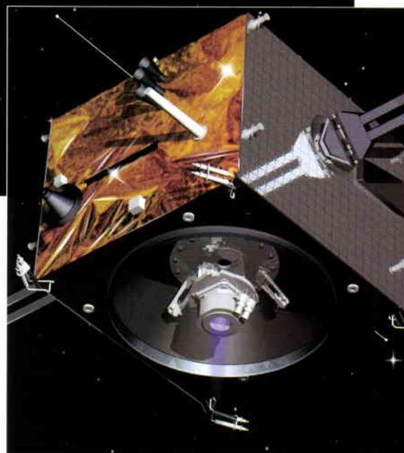
**Figure 5. The SMART-1 satellite being pushed to the Moon by Electric Propulsion (artist's impression courtesy of Swedish Space Corporation)**
