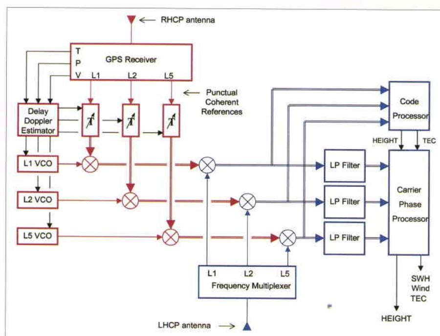
Block diagram of the PIP processor (the processing for only 1 satellite is shown)
