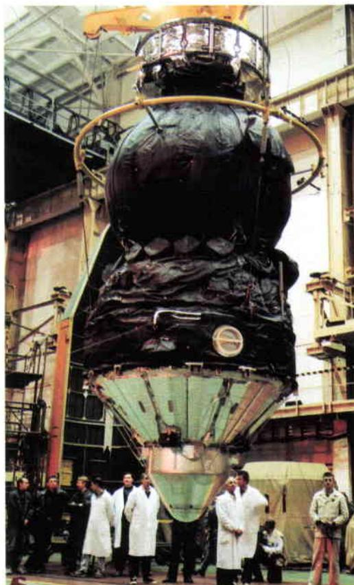
Figure 1. Foton comprises three principal sections: the battery pack (top), the spherical return capsule, and the service module (bottom)
