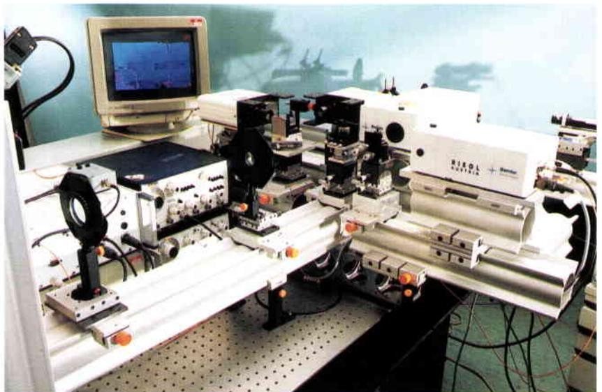
Figure 1. LSPR hardware and experimental set-up
