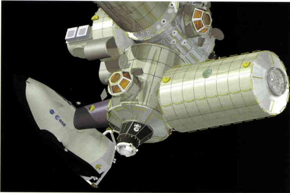
Figure 5. The CRV will remain attached to Node-3 for up to 3 years (ESA/D. Ducros)
