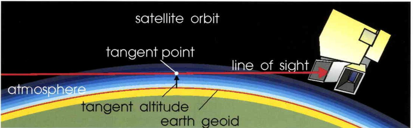
Figure 4. Limb viewing geometry of MIPAS
