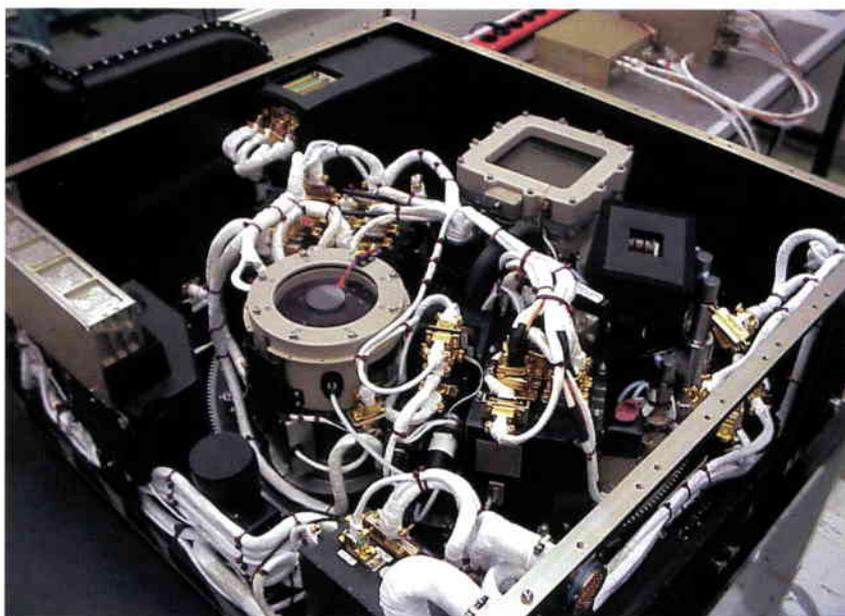
Figure 2. The three Experiment Containers installed on FluidPac's rotating carousel, ready for flight
