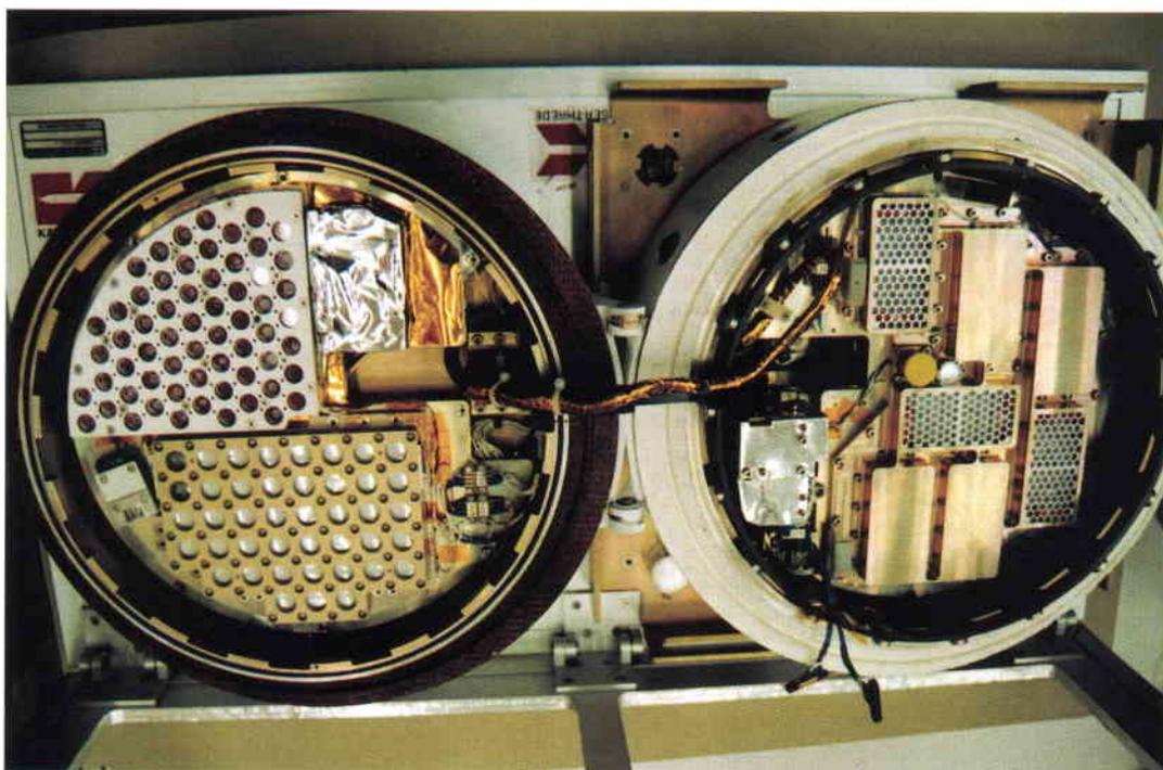
Figure 6. The Biopan experiments integrated on the lid (left) and bottom tray before installation of the thermal blanket. Survival is top left; Yeast is bottom left; Vitamin occupies most of the bottom tray
