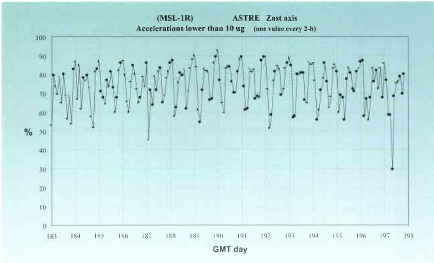
Figure 2. Percentages of the ASTRE data lower than 10 mg along the instrument  $Z_{AST}$  axis ( $X_B$ ) during the whole of mission MSL-1R
