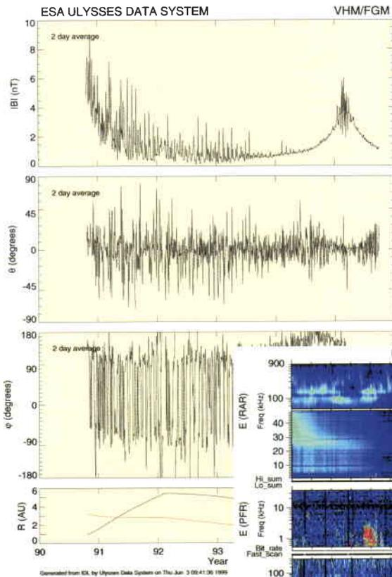
Figure 5. Magnetic-field measurements made by the VHM/FGM experiment on Ulysses during the Solar Minimum Mission. The magnetic field magnitude and components ( $\theta$  and  $\phi$ ) are shown, together with the radial distance from the Sun and the heliographic latitude of the Ulysses spacecraft
