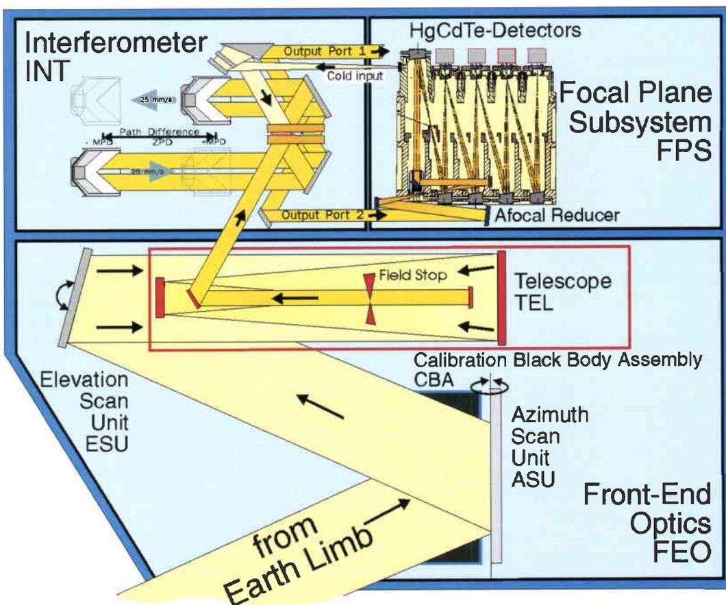
Figure 8. Light path through the MIPAS optics module
