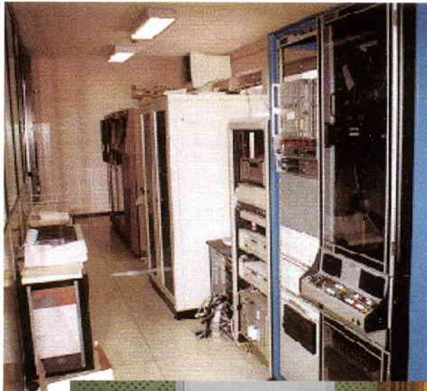
Figure 8. A typical early ground-station computer room with, on the right, a High Density Data Recorder and, at the back, the huge racks of array processors and disks. Today, all of this equipment is replaced by that shown in Figure 9
