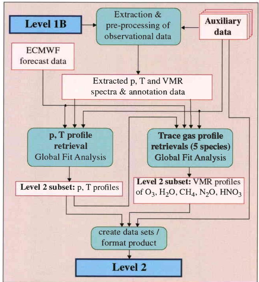
Figure 12. Level 2 processing steps
