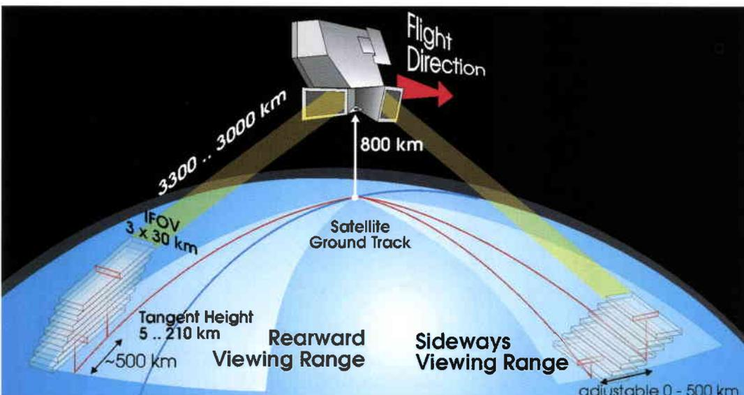
Figure 5. MIPAS observation geometry and rearward and sideways viewing ranges
