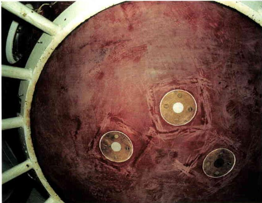
**Figure 7. The three Stone samples installed on the Foton heat shield, close to its stagnation point. The simulated martian sample is at top**
