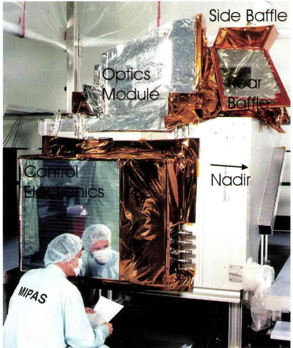
Figure 2. MIPAS instrument during test preparation. In flight, Earth would be to the right
