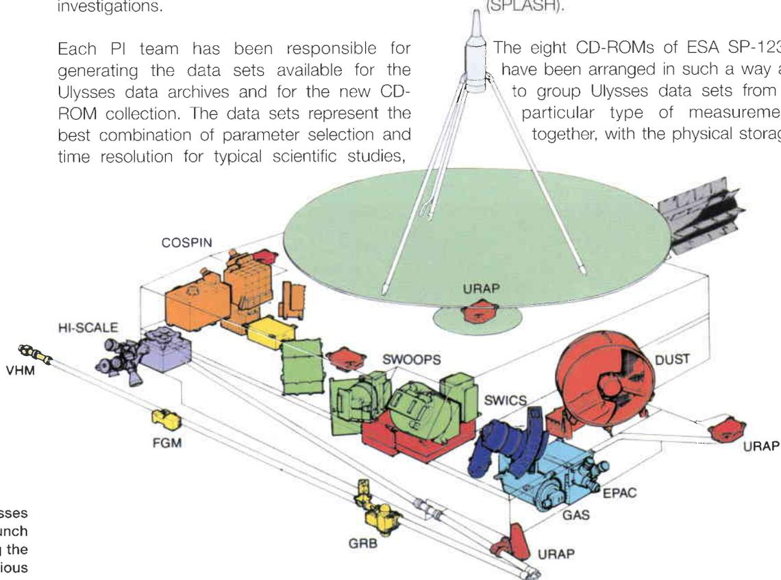
Figure 3. The Ulysses spacecraft in launch configuration, showing the locations of the various instruments
