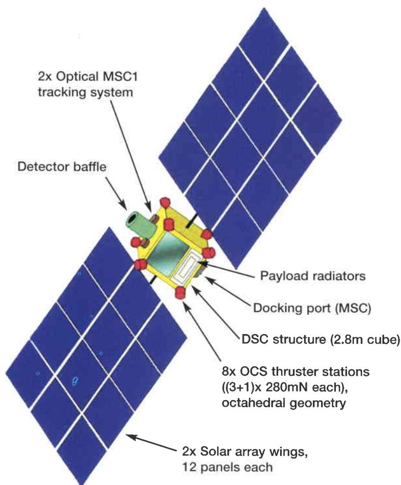
Figure 11. The XEUS Detector spacecraft concept
