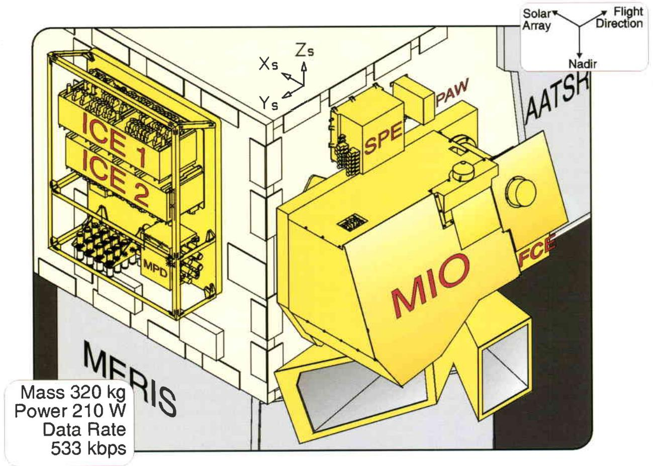
Figure 10. MIPAS mounted on the tip of Envisat
