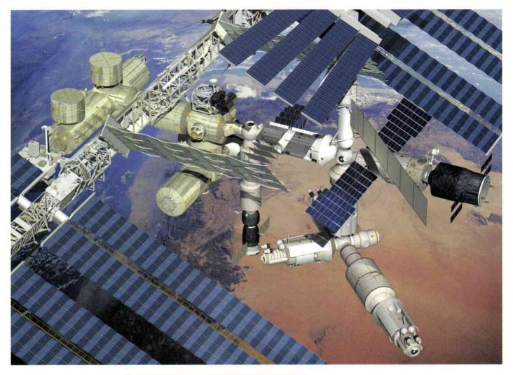
Figure 2. Docked to the Russian Service Module, the ATV is capable of reboosting the ISS into a higher orbit (ESA/D, Ducros)
