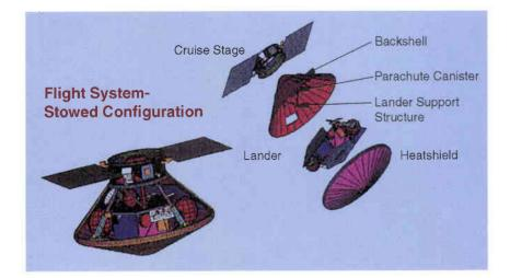
Figure 7. Intermarsnet vehicle configuration
