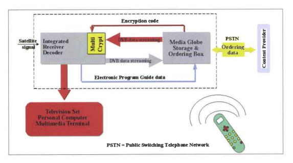
The data are received by the end users via standard satellite dishes (60 cm), possibly with a dual feed for reception from two satellites, and DVB-compatible Integrated Receiver Decoders. The end-user equipment requirements have been established on the basis of the market-analysis and the business-case study. The storage capacity of the end-user equipment is therefore sized according to the expected average use of the system based on the market study.
