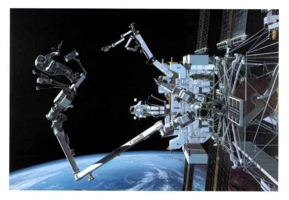
Figure 4. Canada's contribution to the International Space Station, the Mobile Servicing System that will be essential in the assembly, maintenance and servicing of the ISS (photo courtesy of CSA)
