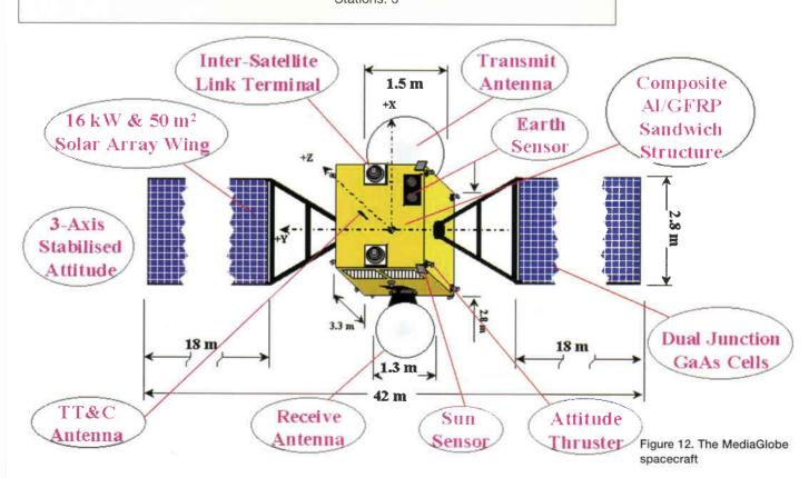
arsenide/germanium solar-panel arrays with nickel-hydrogen batteries. The solar-array performance is 16 kW at end-of-life and the battery capacity is 13 kWh. The spacecraft platform is three-axis-stabilised, with momentum wheels for pitch control and rollyaw stiffness, reaction wheels for momentum storage, and reaction-control thrusters for momentum dumping and attitude manoeuvres.
