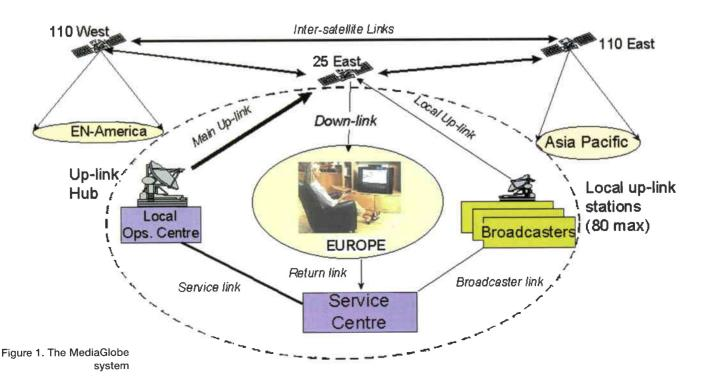
MediaGlobe would be the first space system to allow broadcasters direct access to the satellite and to provide service distribution to three different parts of the World simultaneously.
