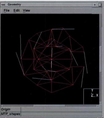
Figure 8. Antenna mode at 53 Hz
