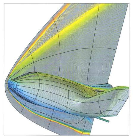
Figure 5. Mach number contours around the X38 (ESTEC)
