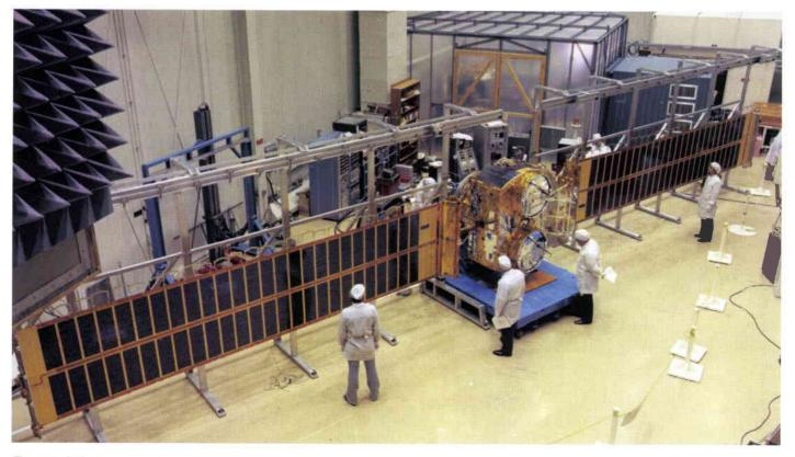
Figure 5. CTS-Hermes engineers monitoring solar-array deployment in the high bay of the David Florida Laboratory, near Ottawa (photo courtesy of Communications Research Centre)
