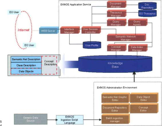
Figure 2. EKNOS architectural concept assigning individual weights to the object relations. Individual weights can be recorded in multi-dimensional matrices for which the indices belong to classes, concepts, object instances and other criteria to be assigned. This technique can boost the precision and performance since it optimises the traversing of search and navigation paths.
