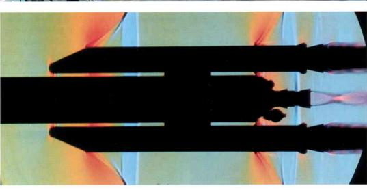
Figure 12. Density contours around the Ariane-5 launcher
