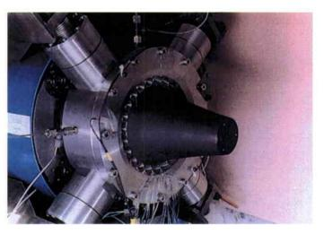
Figure 15. A clustered plug nozzle in the ONERA Ch4 test facility
