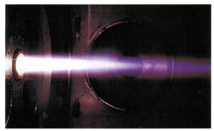
Figure 19. The new 2 MW plasmatron in operation at VKI in Belgium
