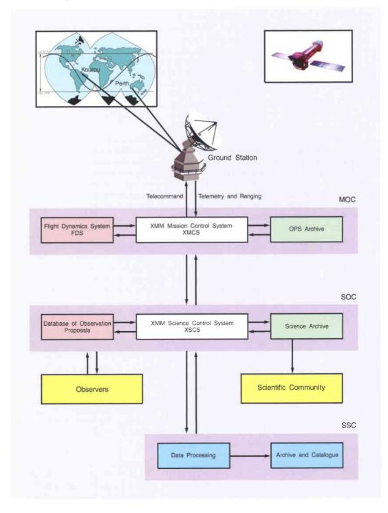
Figure 2. The XMM ground segment
