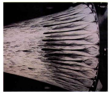
Figure 16b. Oil-film technique measurements (SEP)
