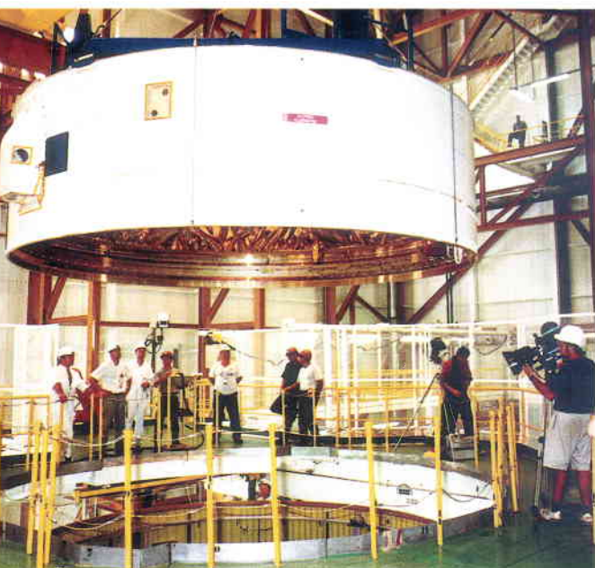
Figure 5. The Vehicle Equipment Bay (VEB). The photograph shows a VEB being mated on top of the main stage in Kourou
