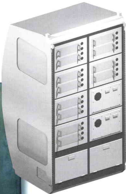
Figure 3. Class 2 payload: European Drawer Rack
