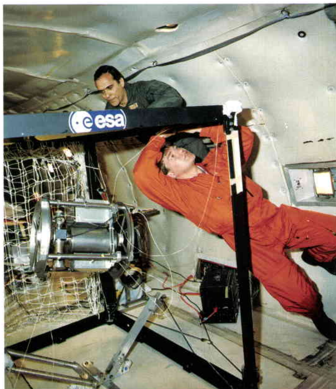
Figure 6. G. Poletti (University of Milan, I) monitoring his experiment on surface forces between contacting solids within a prototype of the Surface Force Assembly (SFA), later flown on Eureka. The equipment is installed in a confining structure with a protective net. (3rd ESA campaign, Mar. 1986) (Photo: NASA)
