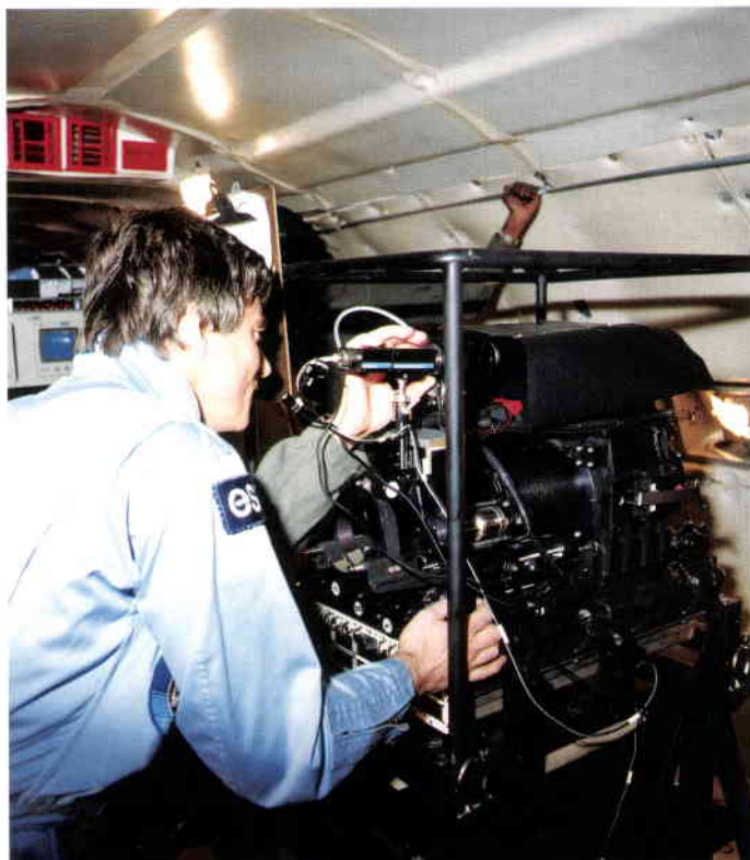
Figure 4. ESA astronaut Ulf Merbold training on the engineering model of the Fluid Physics Module (FPM) (1st ESA campaign, Dec. 1984) (Photo: NASA)
