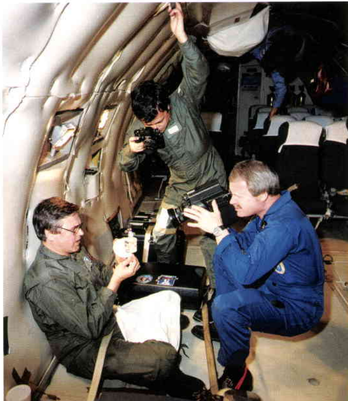
Figure 5. J.C. Legros (University of Brussels, B) performing a test on stability of a fluid interface within a cell, in preparation for his SL-D1 experiment with the FPM (1st ESA campaign, Dec. 1984) (Photo: NASA)
