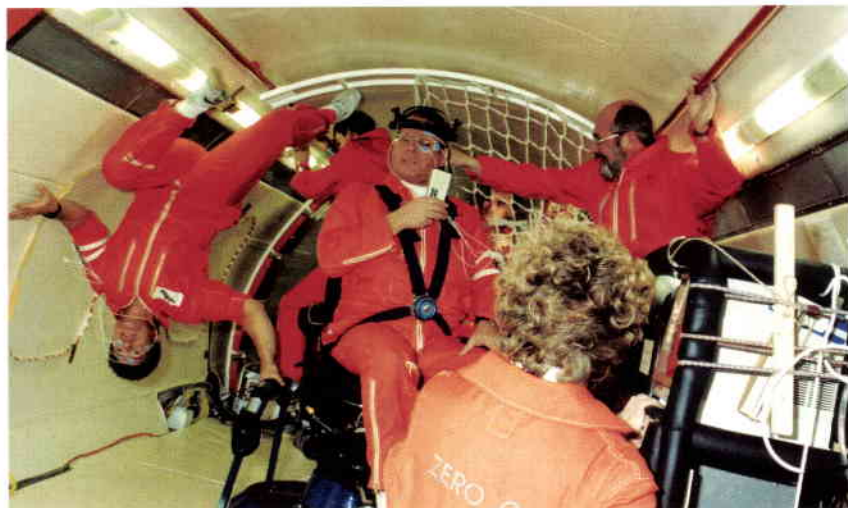
Figure 12. W. Oosterveld (University of Amsterdam, NL), sitting on a rotating chair, is the subject of his own experiment on vestibular rotatory stimulations nystagmus. Eye rotatory motion is recorded by electrodes around the eye. (15th ESA campaign, March 1992)
