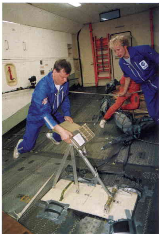
Figure 14. ESA Astronaut Christer Fuglesang, free floating, attempting to sit on the Munich Space Chair designed by E. Pfeiffer (Technical University of Munich, D). The chair allows an astronaut to anchor himself in front of a workstation using feet and thighs, leaving both hands free. (19th ESA campaign, July 1994)
