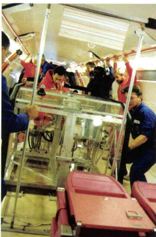
(10) Figure 10. A prototype of the Wet Satellite Model (WSM), the experiment of J. Vreeburg (NLR Amsterdam, NL), being tested in free float. The engineering model of the Advanced Fluid Physics Module (AFPM) in the background is used to rehearse crew handling procedures in preparation for the Spacelab D2 mission. (13th ESA campaign, June 1991)
