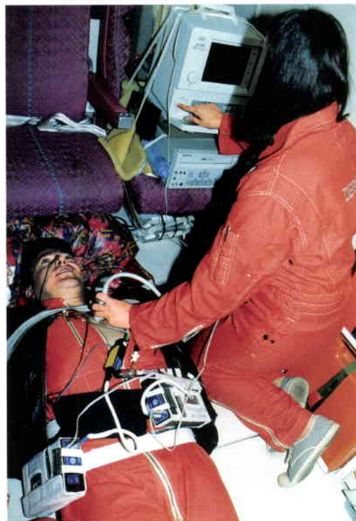
Figure 12. W. Oosterveld (University of Amsterdam, NL), sitting on a rotating chair, is the subject of his own experiment on vestibular rotatory stimulations nystagmus. Eye rotatory motion is recorded by electrodes around the eye. (15th ESA campaign, March 1992)
