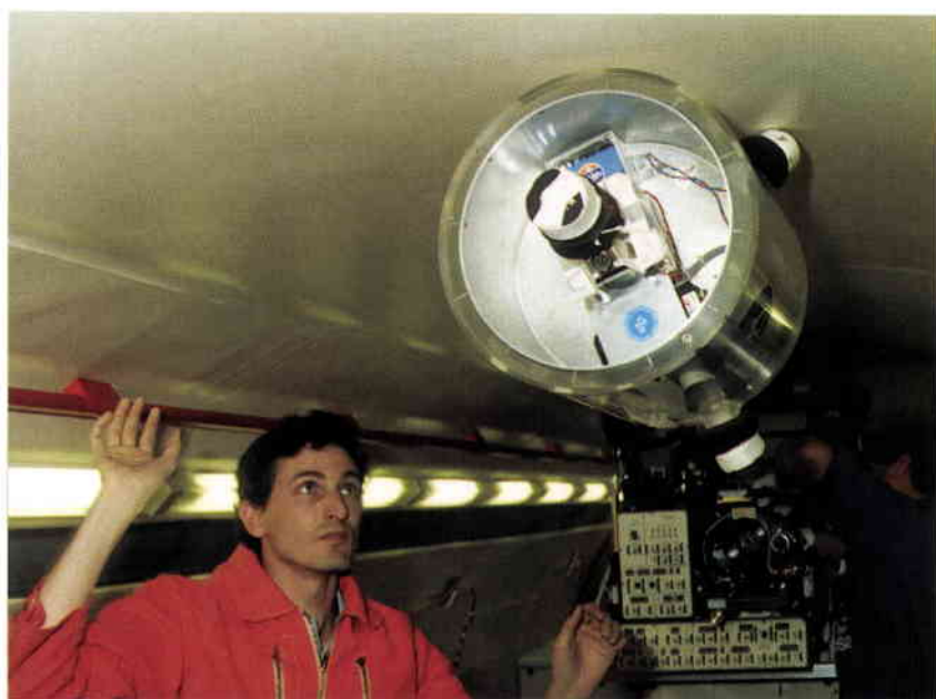
(10) Figure 10. A prototype of the Wet Satellite Model (WSM), the experiment of J. Vreeburg (NLR Amsterdam, NL), being tested in free float. The engineering model of the Advanced Fluid Physics Module (AFPM) in the background is used to rehearse crew handling procedures in preparation for the Spacelab D2 mission. (13th ESA campaign, June 1991)
