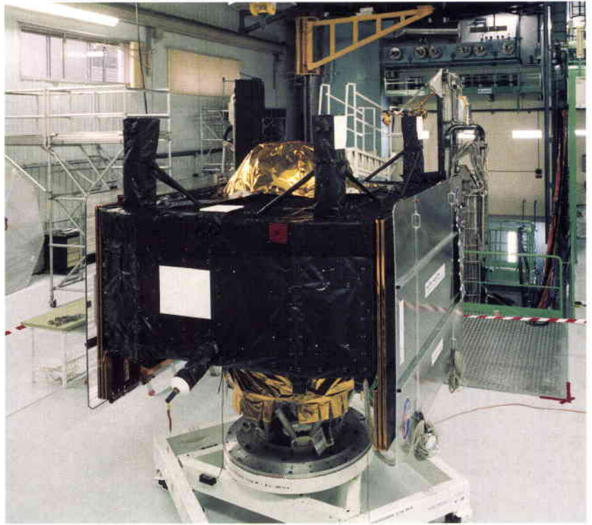
Figure 6. The SOHO service module entering the SIMLES solar-simulation facility at Intespace in Toulouse (F)
