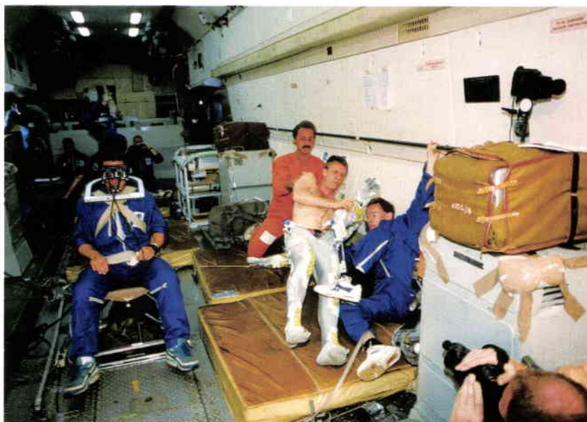
Figure 14. ESA Astronaut Christer Fuglesang, free floating, attempting to sit on the Munich Space Chair designed by E. Pfeiffer (Technical University of Munich, D). The chair allows an astronaut to anchor himself in front of a workstation using feet and thighs, leaving both hands free. (19th ESA campaign, July 1994)
