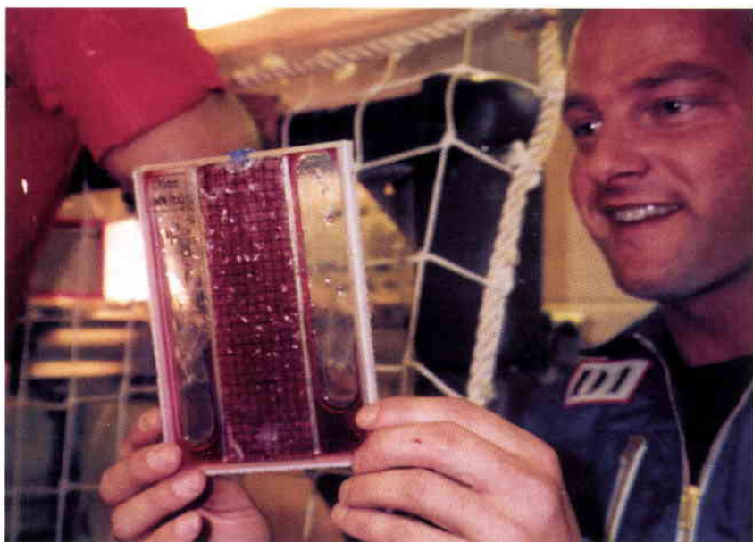
Figure 3. S. Goodman (U of Newfoundland) observing a sample cell during a parabolic flight. In reduced gravity, the fluid in the cell moves up the porous media column by capillary action alone. The experiment is part of research into enhanced oil recovery and contaminant migration in soils, aimed at benefiting the oil and environment industries. (Photo: University of Newfoundland)
