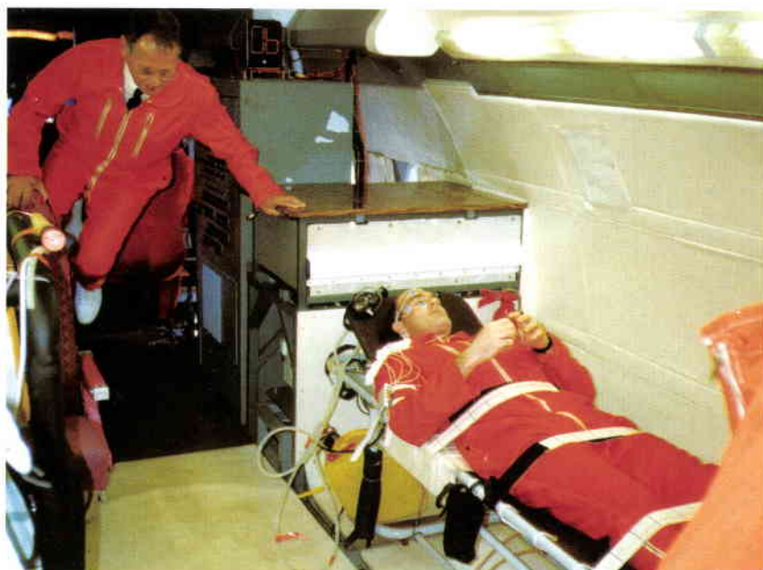
(8) Figure 8. W. Oosterveld (University of Amsterdam, NL) monitoring a subject after injection of hot water (at 44°C) in his inner ear, for an experiment on the vestibular caloric stimulations and nystagmus. Eye rotatory motion is recorded by electrodes around the eye. (11th ESA campaign, Oct. 1990)
