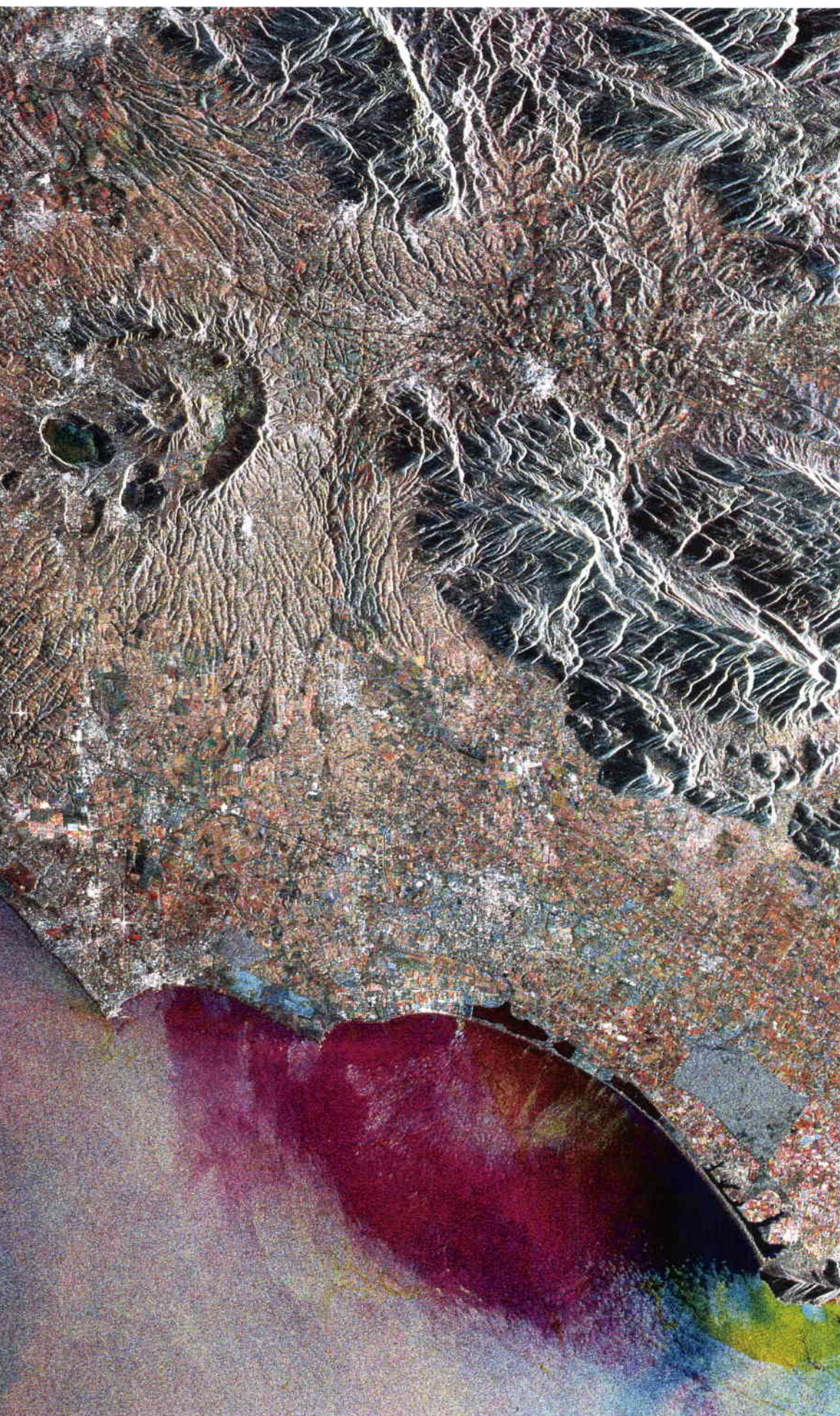
Figure 1. ERS-1 SAR multi-temporal colour composite of the Rome area based on data acquired on 3 January, 6 March and 11 June 1992 by the ESA station at Fucino and processed by ESA/ESRIN in Frascati. Rome is situated top left, while just above the image's centre are the Alban Hills (circular volcanic feature).
