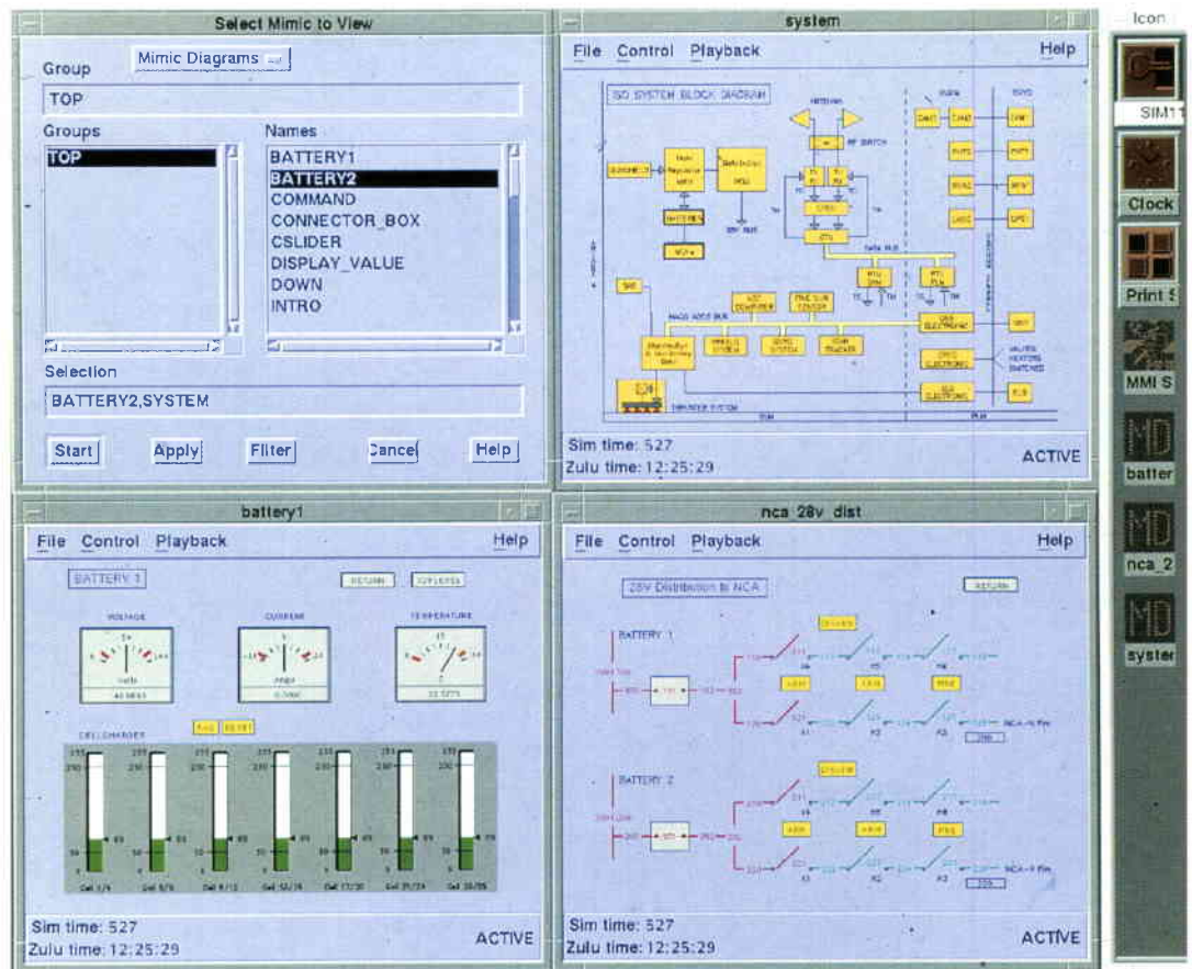
Figure 4. View of the GUI showing synoptic diagrams for: the whole spacecraft (upper right), battery 1 (lower left), and the power distribution to the non-contaminating actuator (lower right) of the ISO simulator. The upper left window allows selection of synoptic diagrams from a library
