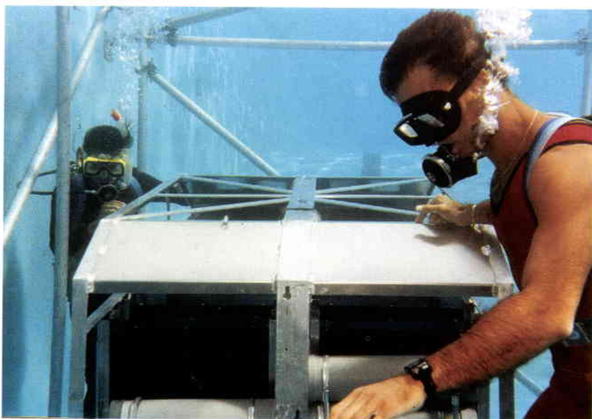
Figure 3. Team members test a rack transportation procedure as part of CIUT-1. The 500 kg mock-up of a rack is lying front-down, and parallel with the central aisle. At the bottom of the photo, three flotation tubes are visible
