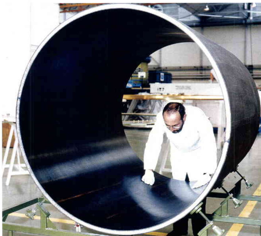
Figure 15. Section of the Polar Platform's central cylindrical structure
