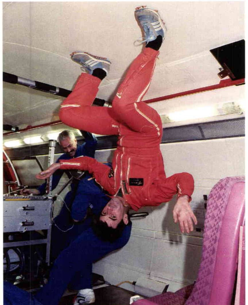
Figure 3. A crew member wearing a prototype of the suction-cup shoe hangs from the ceiling of an aircraft during a parabolic flight
