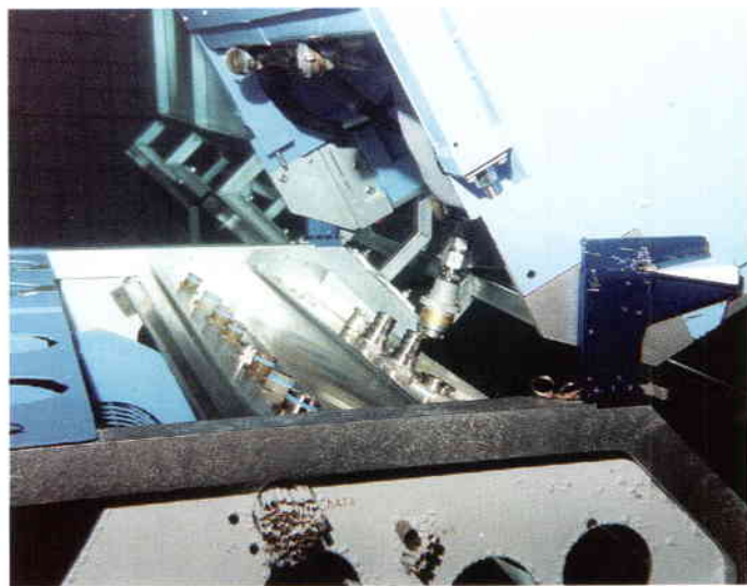
Figure 6. Configuration A hinge, with the hinge pin (behind crew member's head) on the rack and the slotted hinge bracket (in gold) on the stand-off
