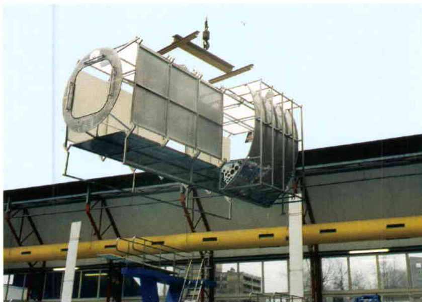
Figure 4. The mock-up of the Attached Laboratory being placed in a swimming pool
