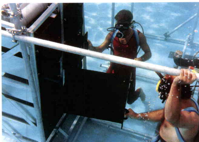
Figure 2. Team members remove a drawer from a lateral rack, while underwater as part of CIUT-1. The rack is installed in a scaffold that represents the central aisle of the Attached Laboratory
