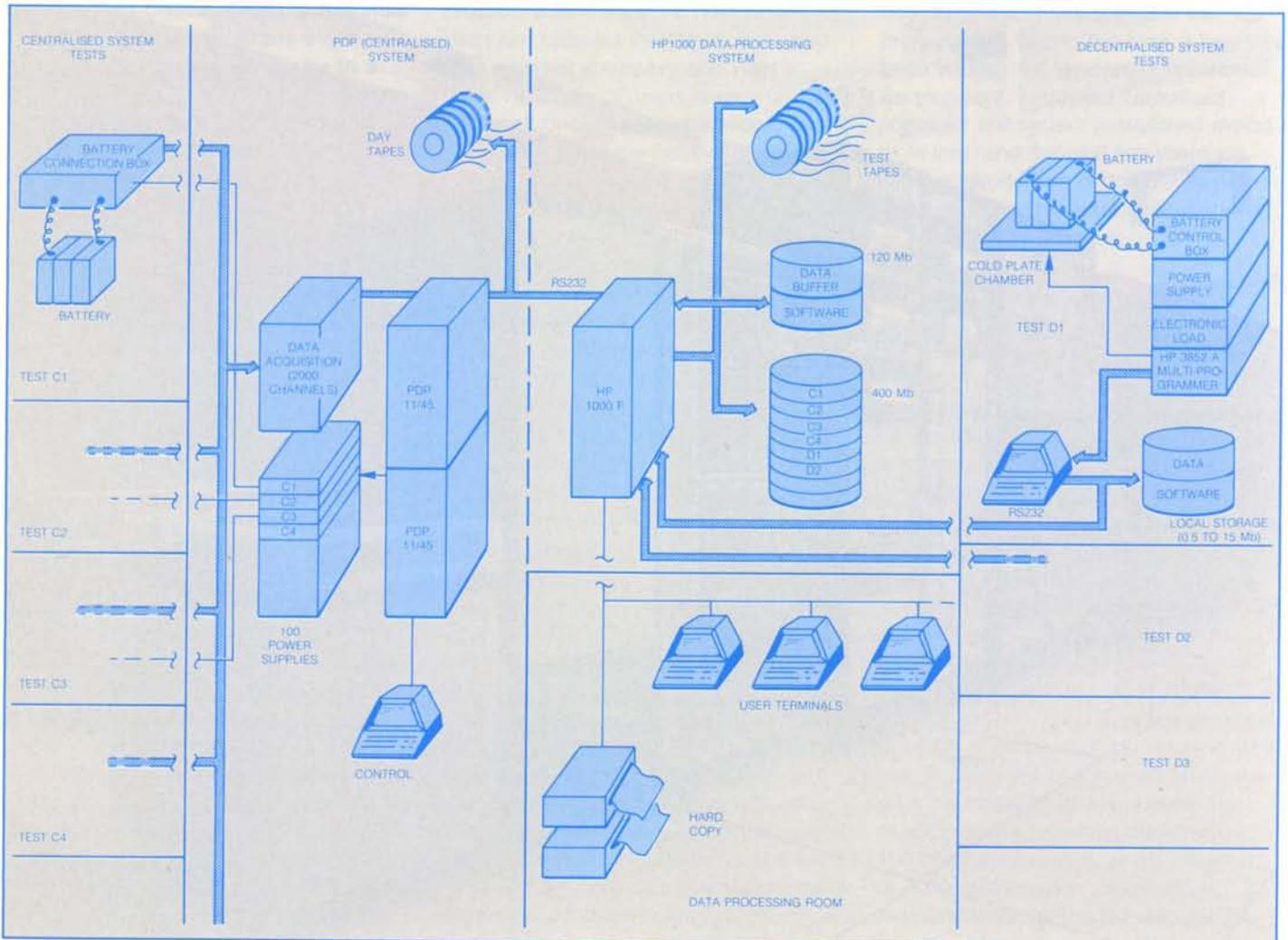
Figure 3 — An 'ELAN' test in progress with batteries in a cold-plate chamber
