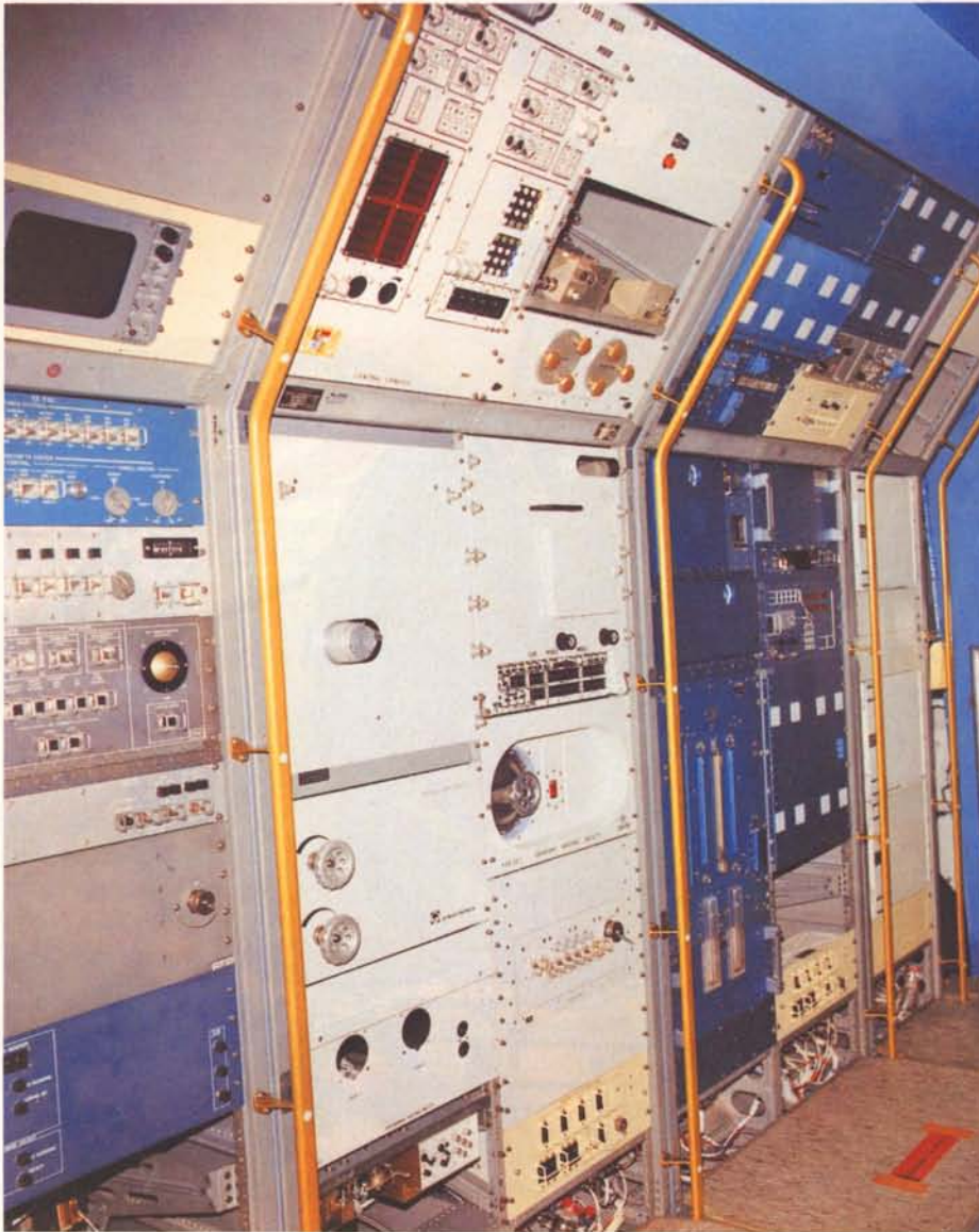
Figure 7 — Spacelab-1's Materials-Science Double Rack (MSDR) photographed at Kennedy Space Center (KSC) in mid-1982
