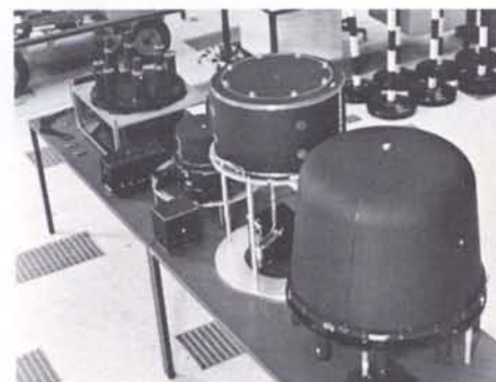
Principal components of Cos-B's central detector package ready for integration. From front to back: anticoincidence dome, energy calorimeter, triggering telescope and associated electronic units
