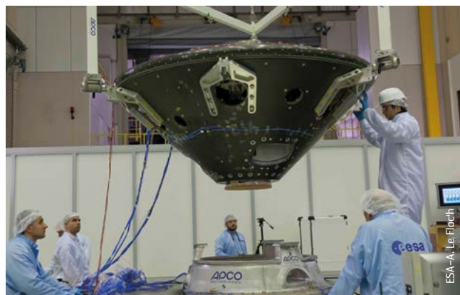
Lowering the 600 kg structural model of Schiaparelli onto the Multishaker at ESA's ESTEC in Noordwijk, the Netherlands, for vibration testing
