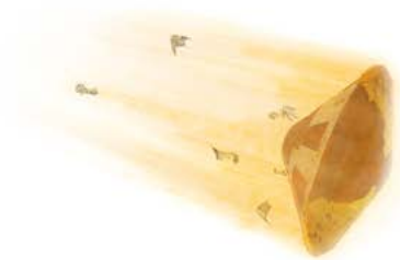
2. Heatshield protects Schiaparelli during deceleration in atmosphere
