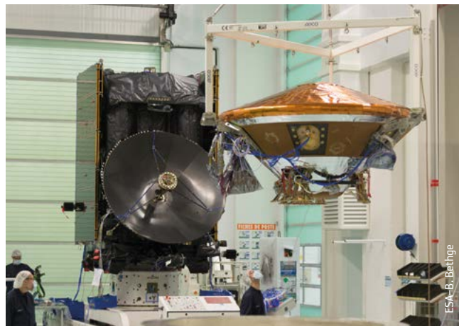
Schiaparelli being craned into position for mating with TGO in the Cannes facility of Thales Alenia Space (France)
