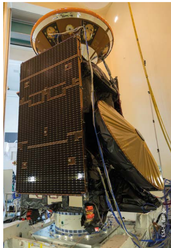
TGO with Schiaparelli (top) during testing at Thales Alenia Space, in Cannes (the high-gain antenna is on the right)
