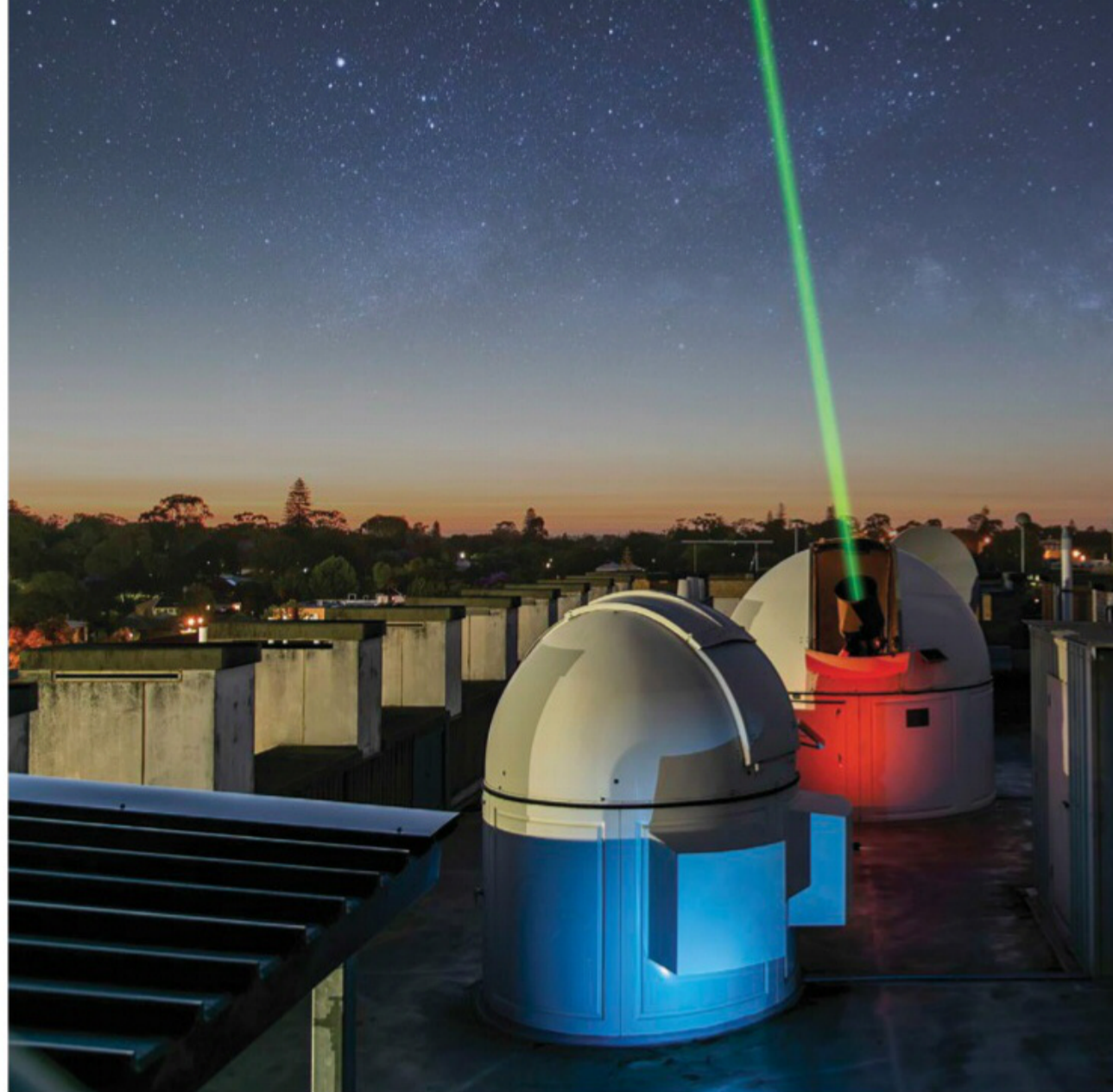
UWA’s rooftop observatory telescope dome containing one of the self-guiding optical terminals which can be used for more stable and high-speed optical communications.
