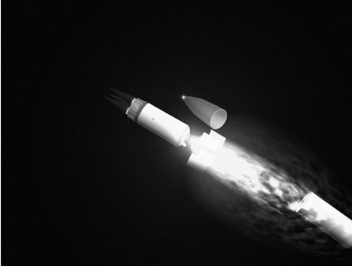
**Minuteman launch sequence.** The Minuteman III third stage produces sufficient thrust for the RV bus to put it into a proper ballistic flight path. The warhead's protective cover is jettisoned to reveal three RVs. (Courtesy, U.S. Air Force)
