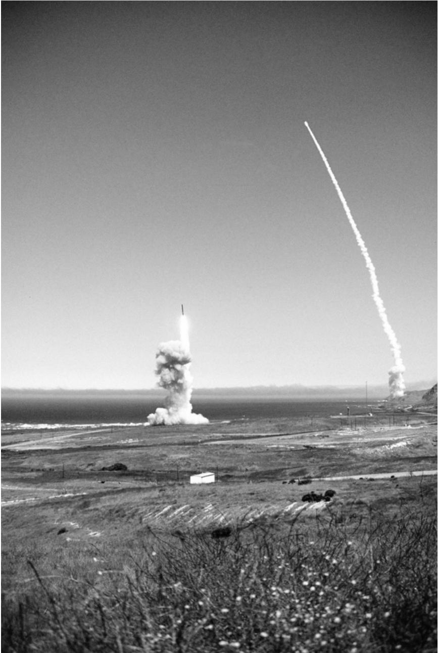
**Minuteman dual launch.** Solid fuel-powered ICBMs like these Minuteman III missiles begin launch operations with the ignition of its first stage within its silo. A Minuteman III launch crew controls up to ten missiles. (Courtesy, Department of Defense)
