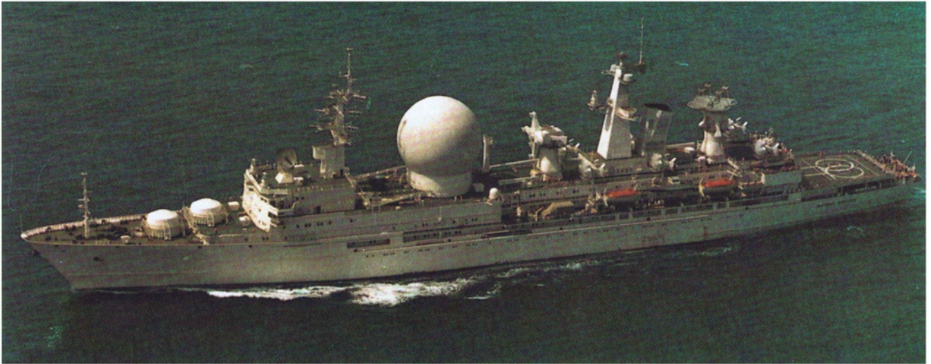
Shown here is the AGI MARSHAL NEDELIN, lead ship of the newest class of Soviet space support ships, equipped to support spacecraft launch and recovery, and manned space activity. These ships provide additional mobile monitoring, data relay, and communications, extending the Soviets' ability to monitor their satellites beyond their homeland.
