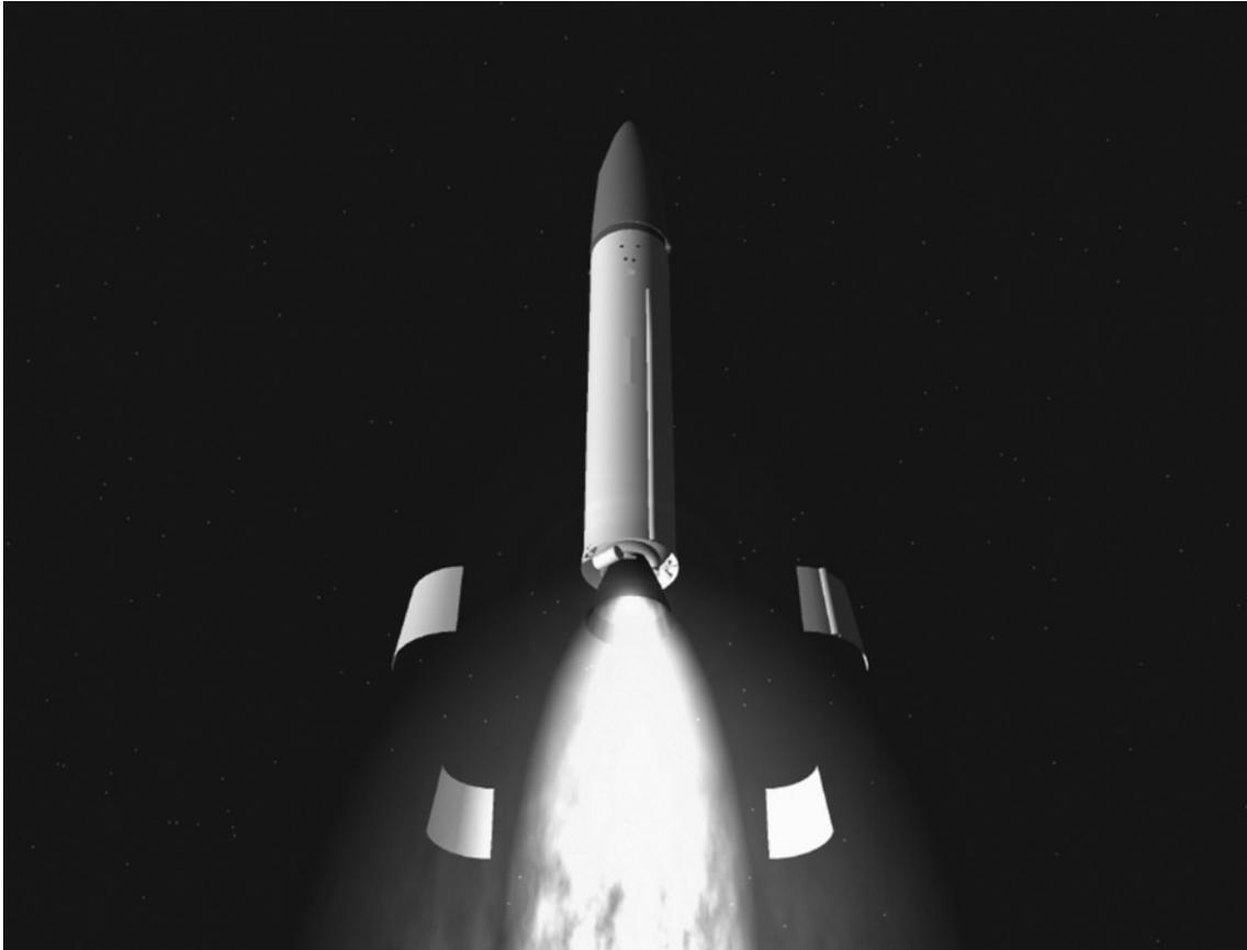
**Minuteman launch sequence.** After the first-stage ignition, the Minuteman III completes its boost phase with its second-stage rocket motor “burn” that increases the missile’s velocity. (Courtesy, U.S. Air Force)
