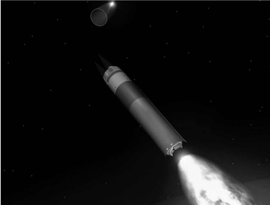
**Minuteman launch sequence.** During second-stage flight, the Minuteman III prepares for its mid-course phase by shedding its warhead's nosecone. The second stage's solid fuel is almost spent and it will soon separate from the remaining components. The Minuteman can travel upward to 6,000 miles. (Courtesy, U.S. Air Force)
