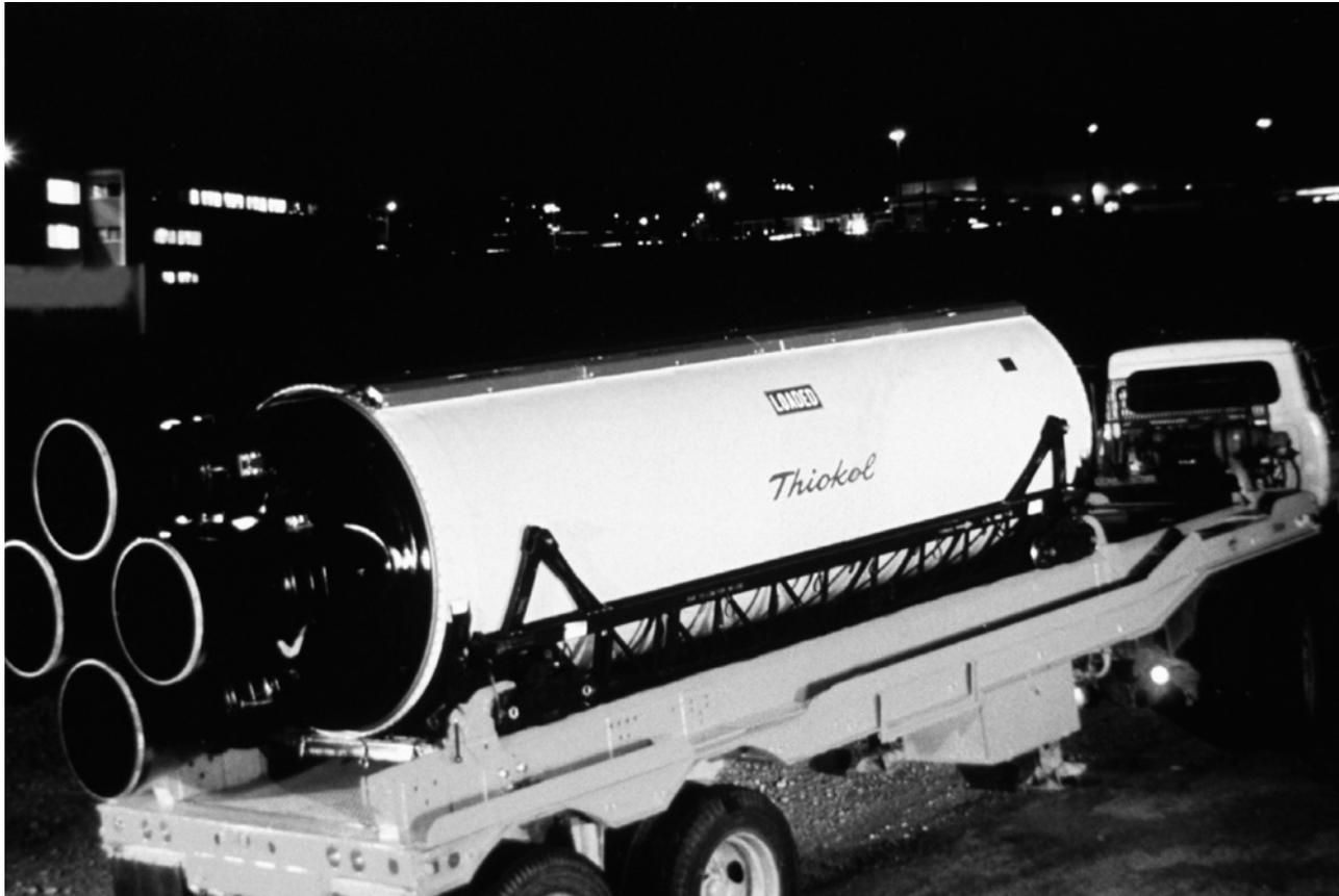
**Minuteman first stage.** The United States converted its land-based ICBMs from liquid to a majority solid fuel-based force. The Minuteman's first stage used four combustion chambers to power it into flight. (Courtesy, Department of Defense)
