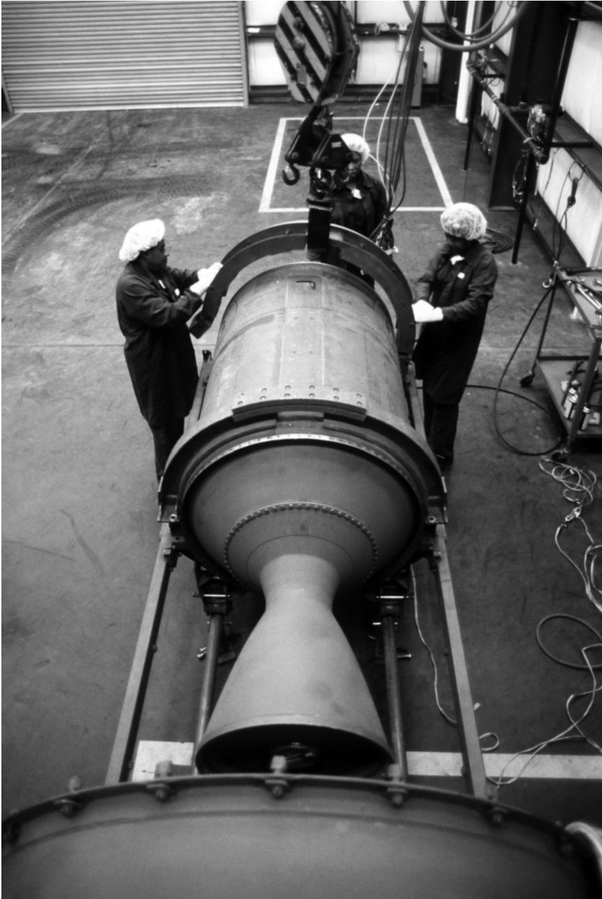
**Pershing I second stage.** Combustion chambers must withstand intense temperatures and pressures when the rocket motor or engine operates. This Pershing I solid fueled rocket motor illustrates a typical combination chamber that concentrates the rocket exhaust to increase thrust. (Courtesy, Department of Defense)
