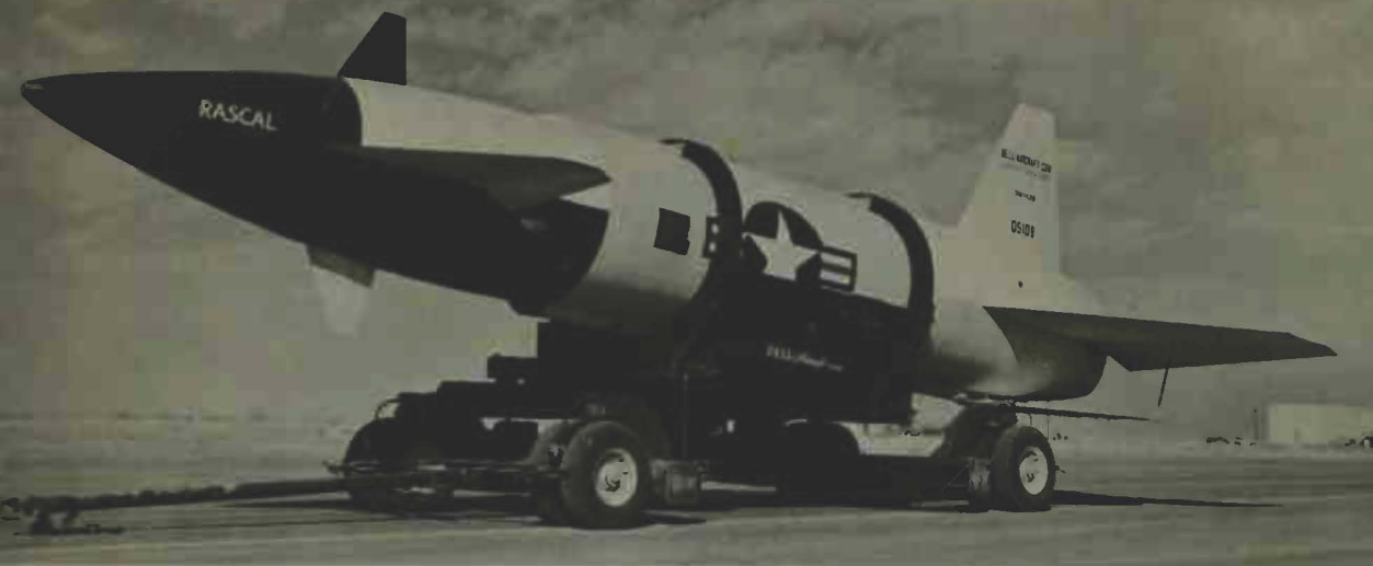
GAM-63 Rascal air-to-ground supersonic missile on DUC carrier. The rocket-propelled missile is built by the Bell Aircraft Corp., Buffalo, N. Y.
