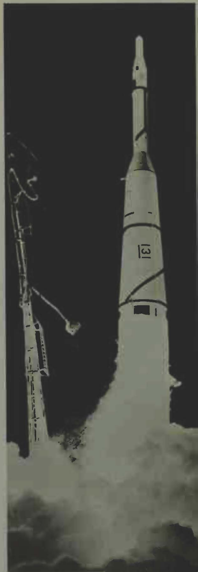
Discoverer VII is prepared for launch from Vandenberg Air Force Base, California. The Agena satellite vehicle used in Project Discoverer is boosted into polar orbit by an intermediate-range ballistic missile.
