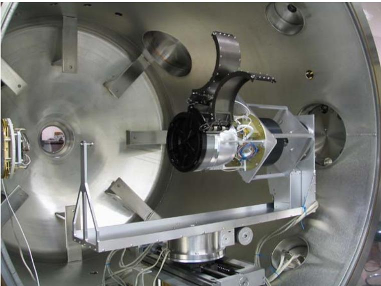
Fig. 27 SWAP instrument mounted on four-axis positioning system
