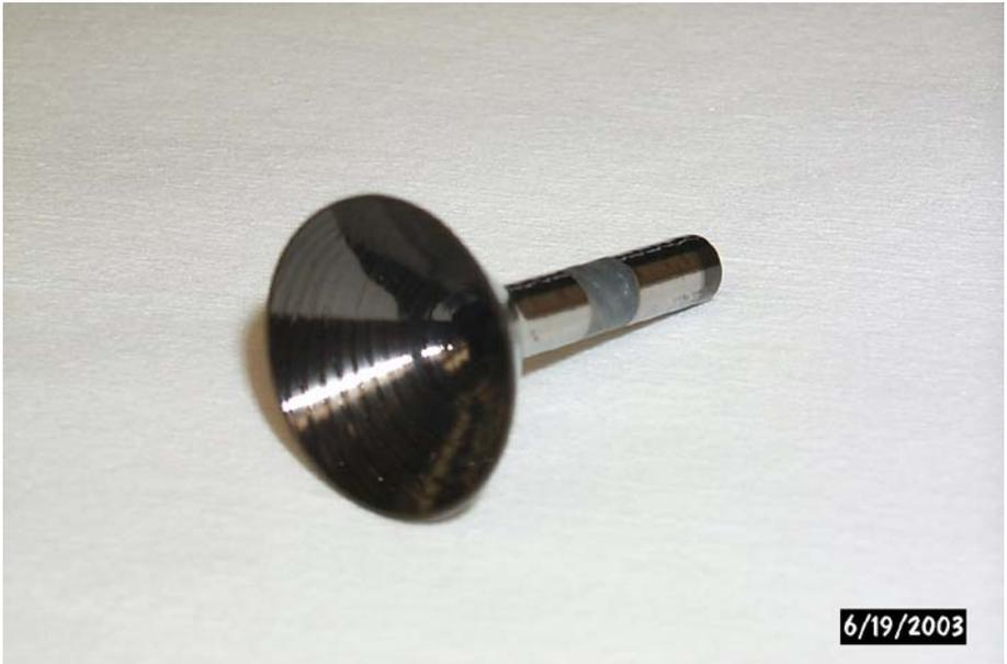
Fig. 16 Quad spiral channel electron multiplier
