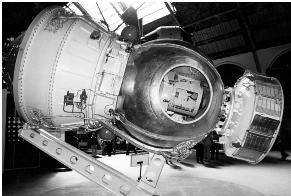
This mock-up of a later Bion capsule (Bion 6) shares the same basic configuration as the capsule used on the early Bion flights. (Photo: State Scientific Centre of Russian Federation, Institute for Biomedical Problems of the Russian Academy of Sciences)
