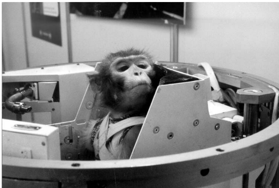
Monkey in a Bion flight capsule. This same design was used for all of the Bion monkey flights, Bion 6–12. (Photo: State Scientific Centre of Russian Federation, Institute for Biomedical Problems of the Russian Academy of Sciences)
