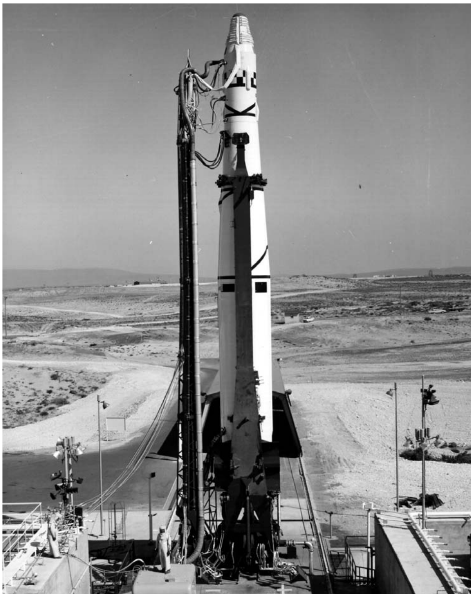
The Thor-Agena combination used in Discoverer launches. (Photo: USAF)
