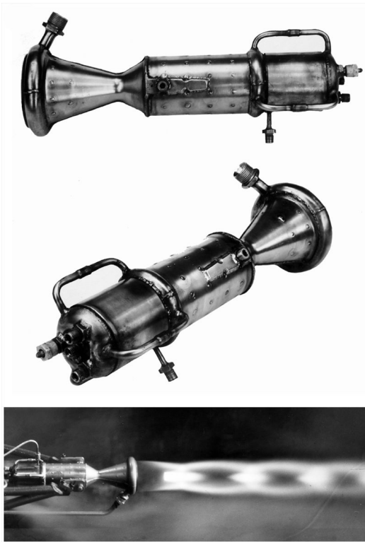
Figure 59. The third stage would have been powered by the PR.38 motor. Here a chamber for that motor is being test fired.
