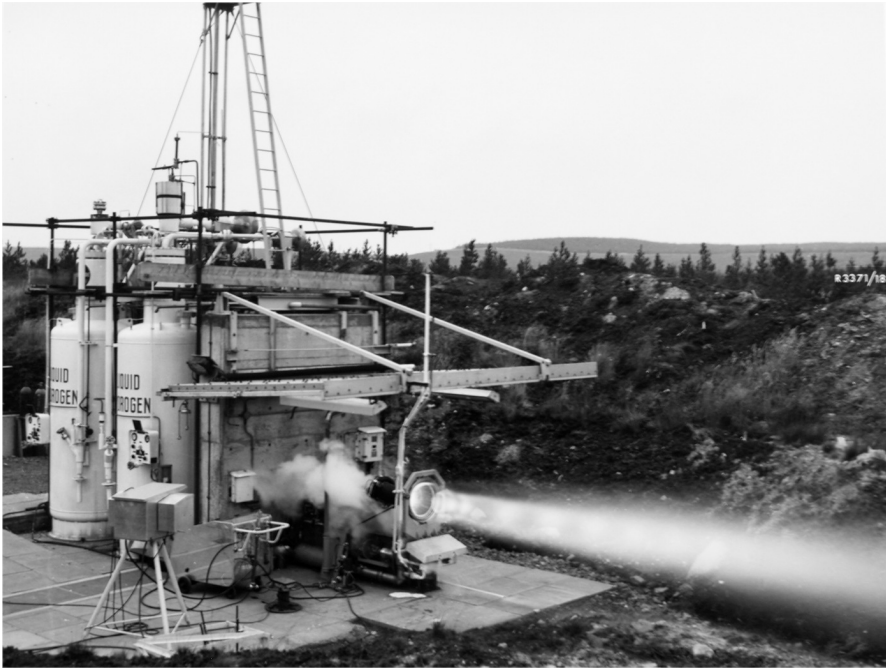
Figure 19. Rolls Royce RZ 20 hydrogen motor being test fired at Spadeadam.
