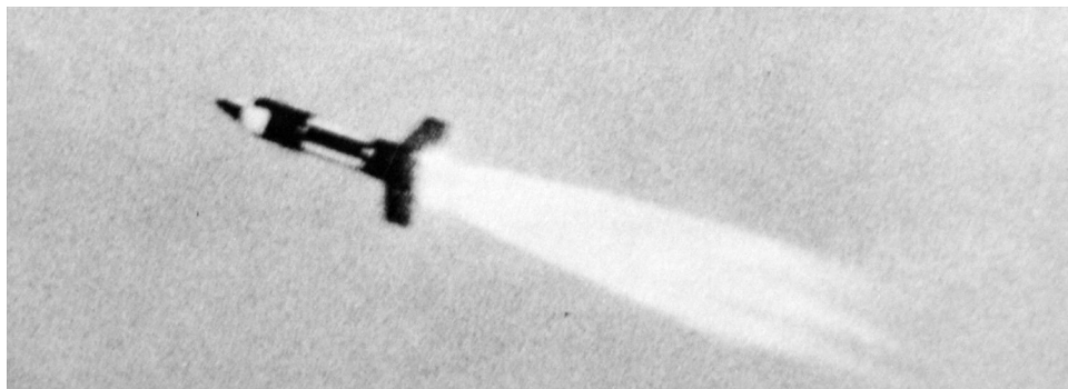
Figure 85. Base drag test vehicle in flight.
