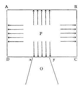
Assume a chamber ABCD, walled solidly on all sides. An explosion takes place within it, building up pressure, P. According to our knowledge of the behavior of gases under pressure, the gas
