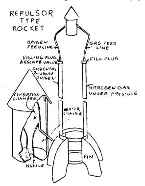
This Mirak would have been able to fly upward with an initial acceleration of more than 32 feet per second per second. It carried enough fuel for about thirty seconds of burning, and would have been sapable of reaching a height of three miles or better. But unfortunately there seemed no simple way of equipping it with a parachute apparatus to bring it back safely, and without a parachute it would have been smashed on its first flight.
