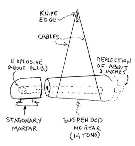
NOTE: CHARGE IS SET OFF BY ELECTRICITY, AND THE SWING OF THE PENDULUM IS MEASURED.
