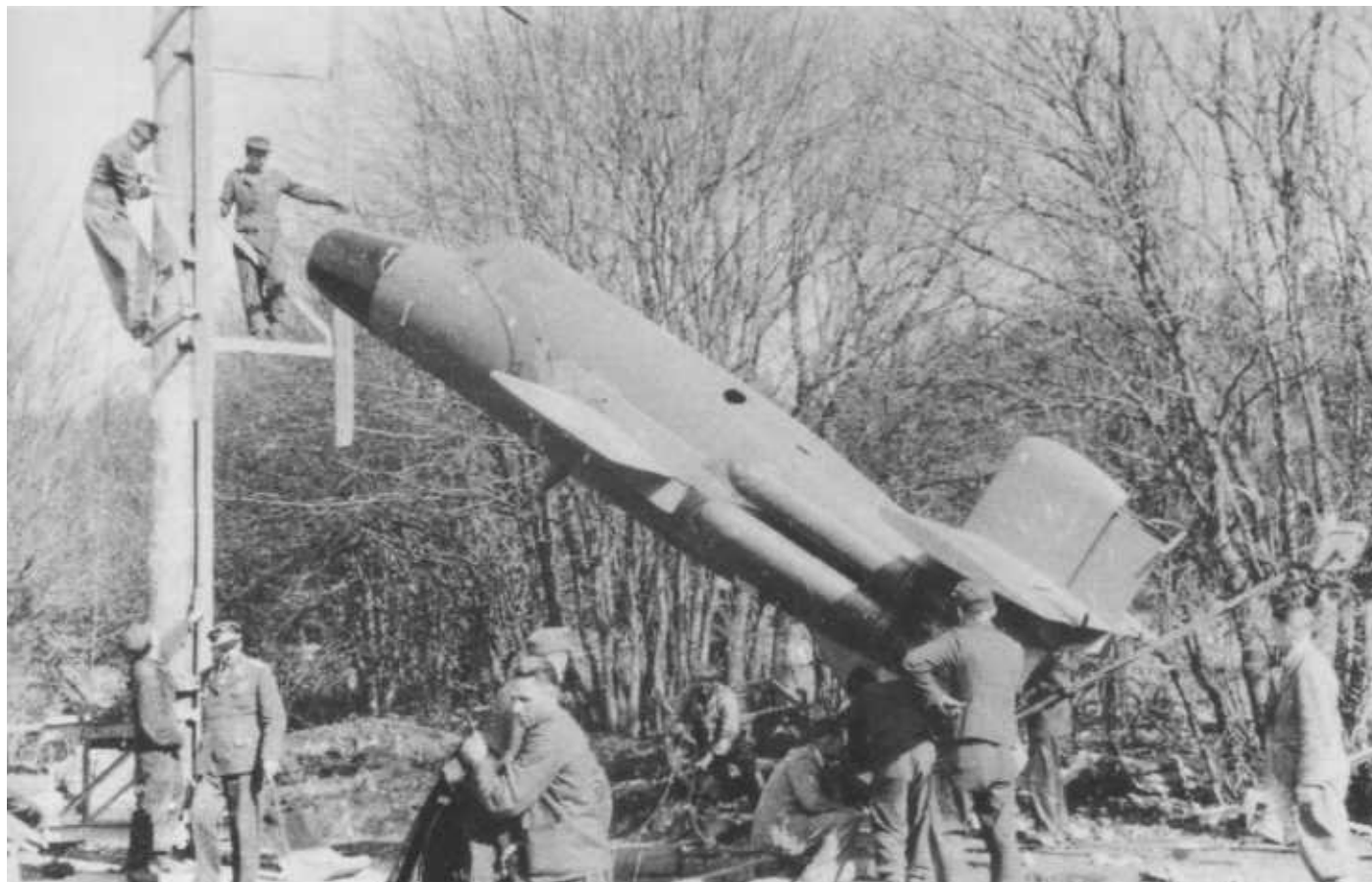
The " Natter ," as seen from its port side, has been lifted off of its cradle and Bachem Werke personnel are man-handling the 349A to bring it vertical along side the pine pole.
