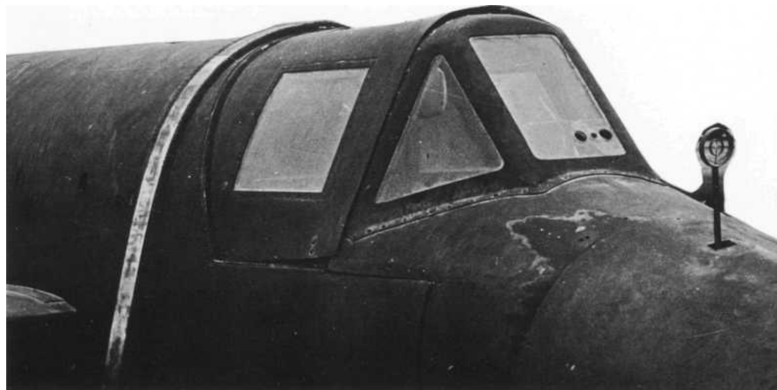
A close up of the T2-1011 at Freeman Field showing its round ring sight for aiming its 24 R4M rocket shells into an Allied bomber formation.
