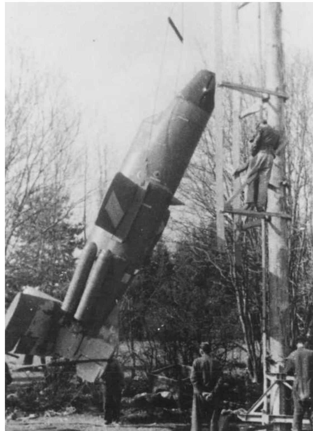
In this view we see the starboard side of the " Natter " being lifted up to be secured to the pine tree pole launcher. Underside the starboard wing appears a painted on "dash" to track it visually after lift-off.
