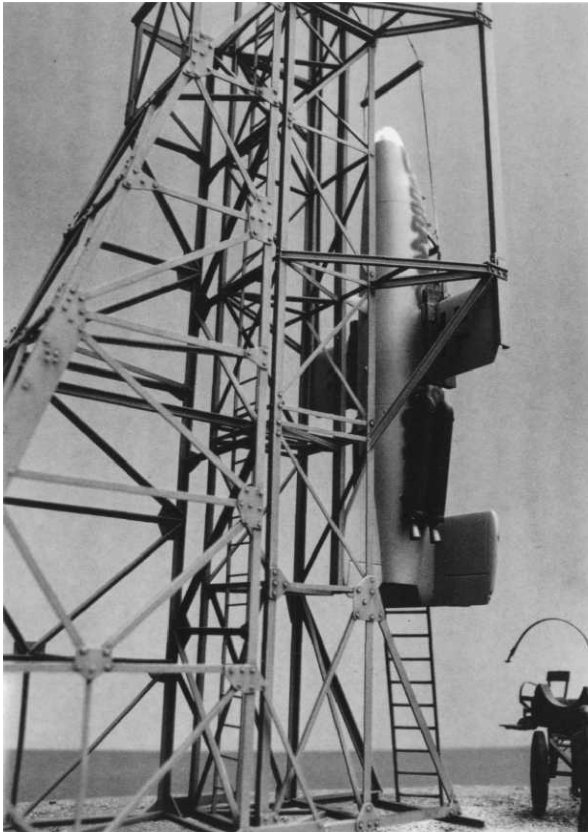
The port side of a Ba 349A mounted on its metal frame launch ramp. Notice the paired Schmidding 533 booster rockets in black camouflage. Scale model by Reinhard Roeser .
