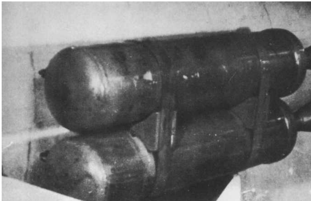
Another view of a Ba 349A 's port side Schmidding 533 booster rocket engines.
