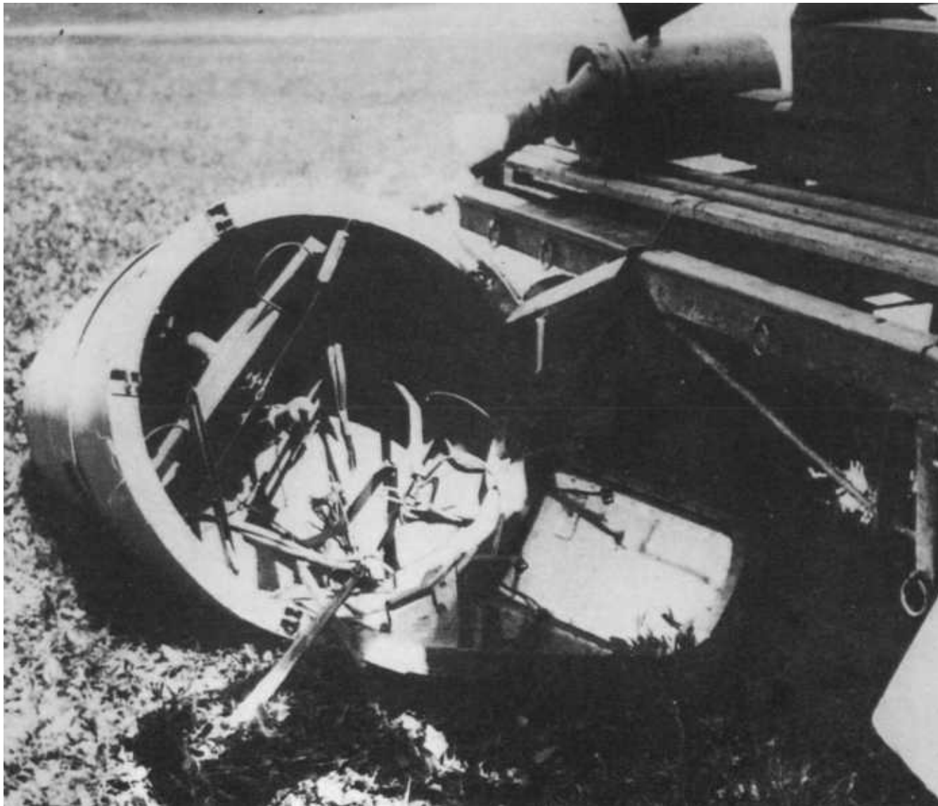
The object in this photo appears to be the entire upside down nose section from a Ba 349A . Rudder foot pedals can be seen at the top of the object along with other miscellaneous cables. This nose section was also found at St. Leonard, Austria.
