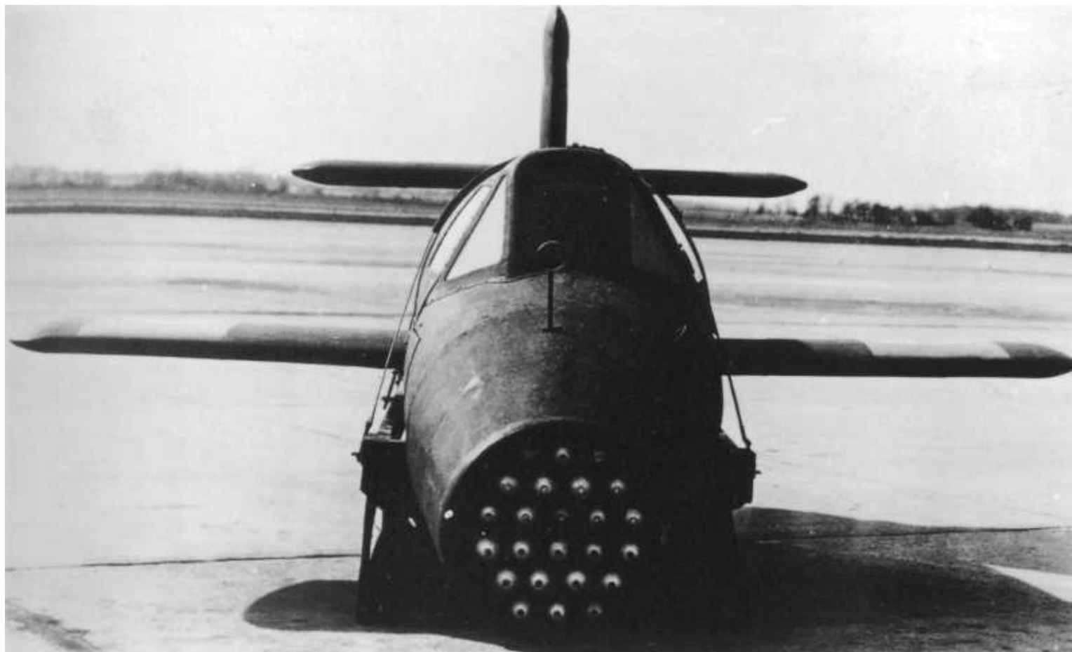
A direct on nose view of the Ba 349A with its twenty four R4M rocket shells as seen at Freeman Field post war. The battery of rockets were aimed by a crude ring sight which can be seen a few feet aft the Ba 349s nose.
