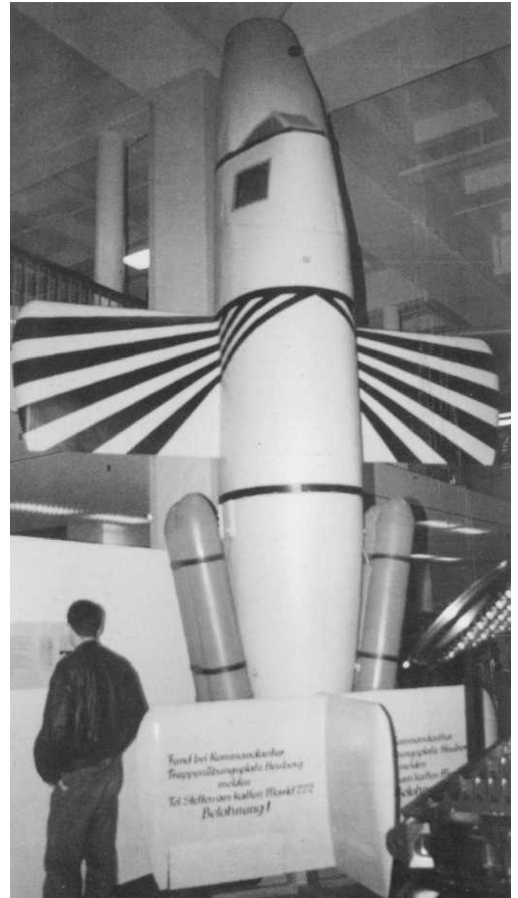
The Deutsches Museum's M-17 painted Ba 349 . The size of the M-17 (small) can be judged by the man standing near its port side Schmidding 533 booster rocket and the port side elevator. Photographed by Gary Hethcoat.
