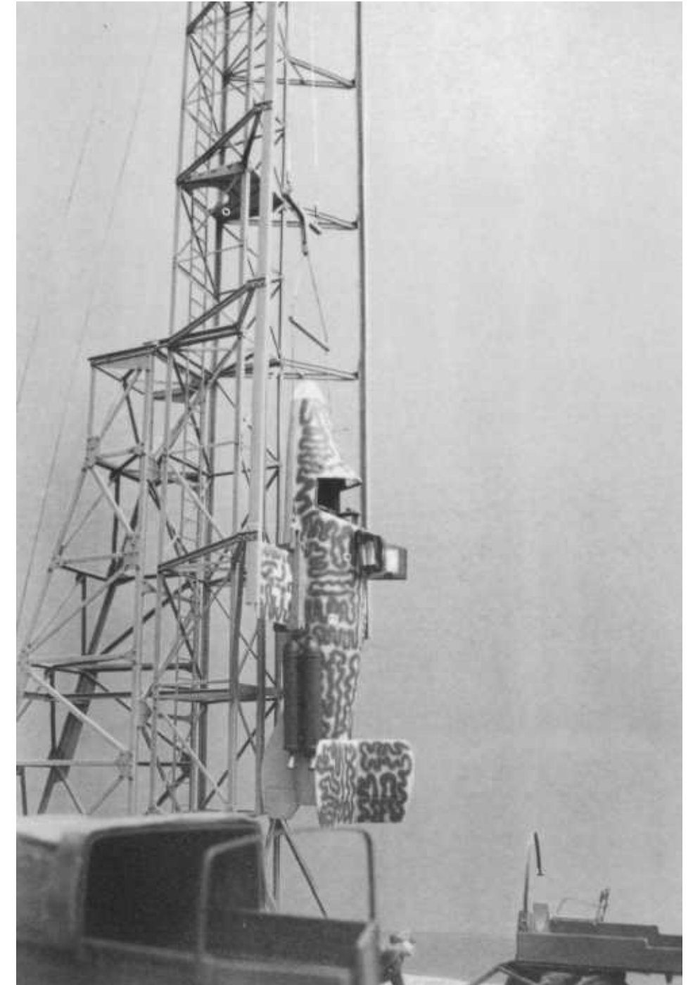
It appears that a spreader bar with two cables are used to haul the " Natter " (a Ba 349A shown on the tower) up on the metal frame launching ramp. Scale model by Reinhard Roeser .
