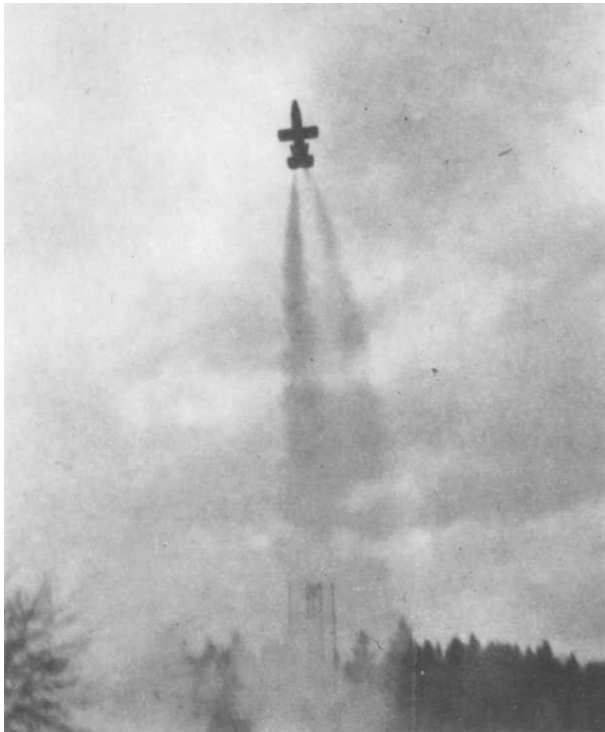
Above: Lift-off of an unmanned 349 during Bachem's initial flight testing program. At the beginning several unmanned " Natters " failed even to clear the metal frame launch tower. The reason was due to the differential thrust provided the 4x Schmidding 533 booster rocket engines. After much trial and error the booster rockets became better coordinated.
