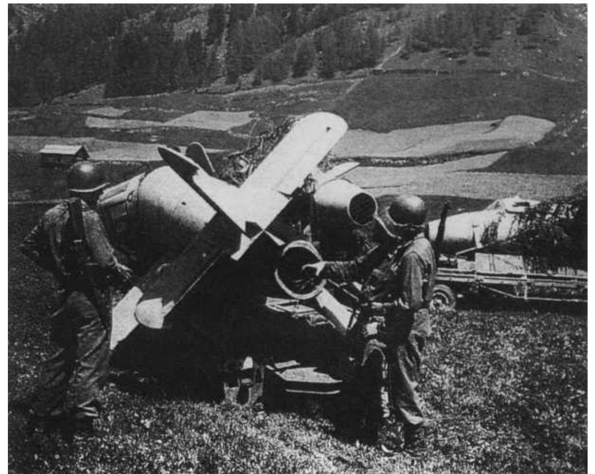
Another view of one of the ten Ba 349A s found at a mountain top site near St. Leonard, Austria. The American GI is pointing to the exhaust orifice of the HWK 509 's bi-fuel rocket engine. The nose of another Ba 349A is to the immediate right and shows empty R4M 73 mm rocket rack.
