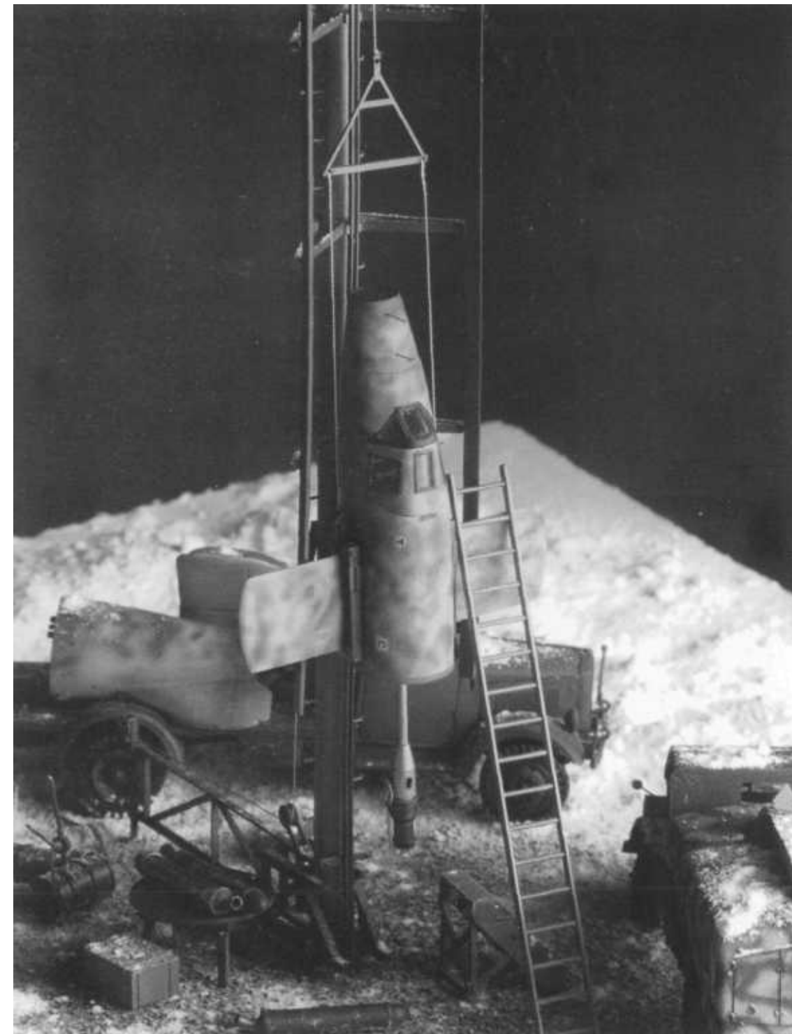
The M-23 , giving a good view of its HWK 509 thrust tube and combustion chamber, is shown mounted on a pine tree pole launcher. Its tail assembly is on the 2 1/2 ton Henschel truck. Notice the cluttered burnt ground around the launch site. Its cluttered with spent Schmidding 533 solid fuel rocket booster engines. Scale model and photographed by Jamie Davies .
