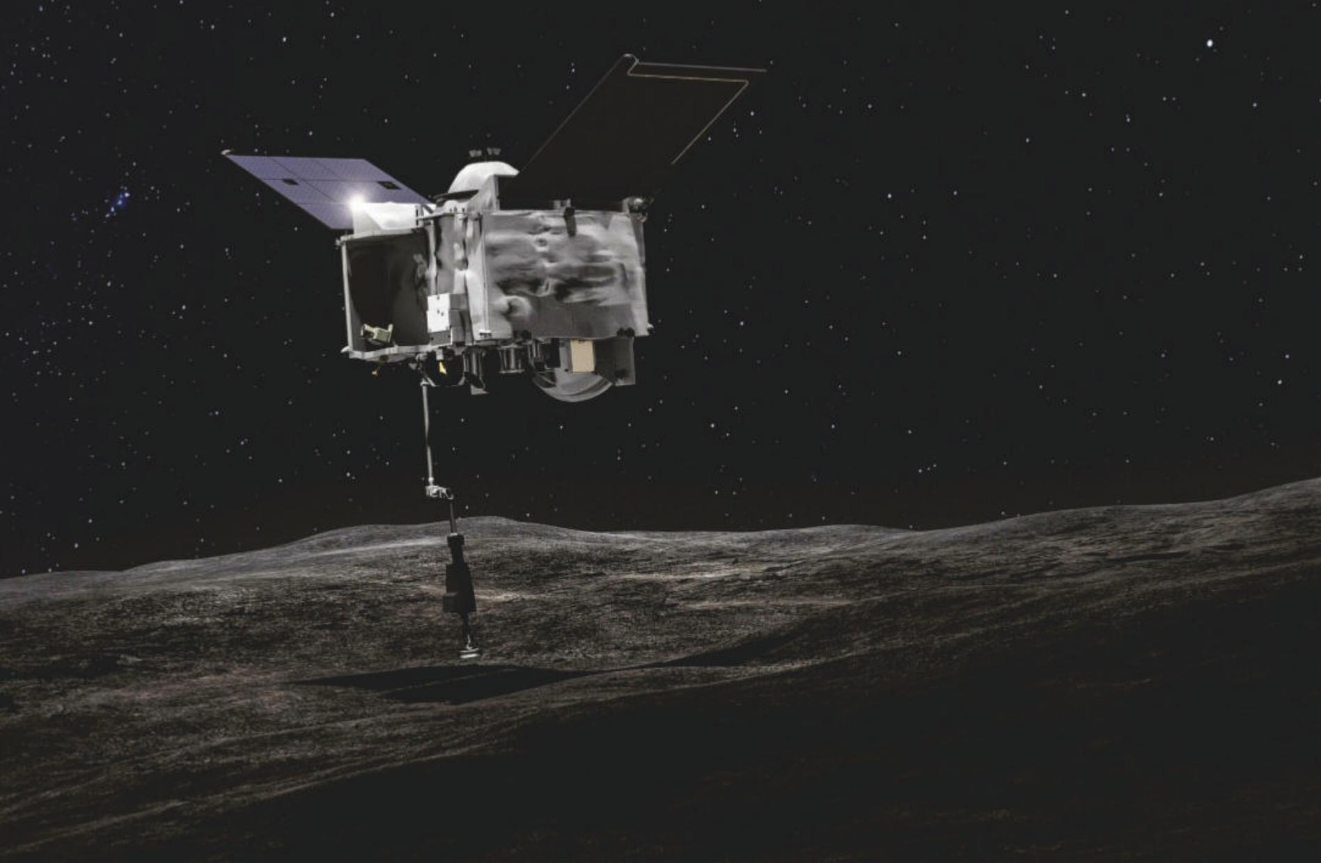
↑ An artist's rendering of the procedure Osiris-Rex will use to collect a sample of Bennu: Hover just above the asteroid's surface while a robotic arm extends to blow on the regolith and bag up to four pounds of gravel.
