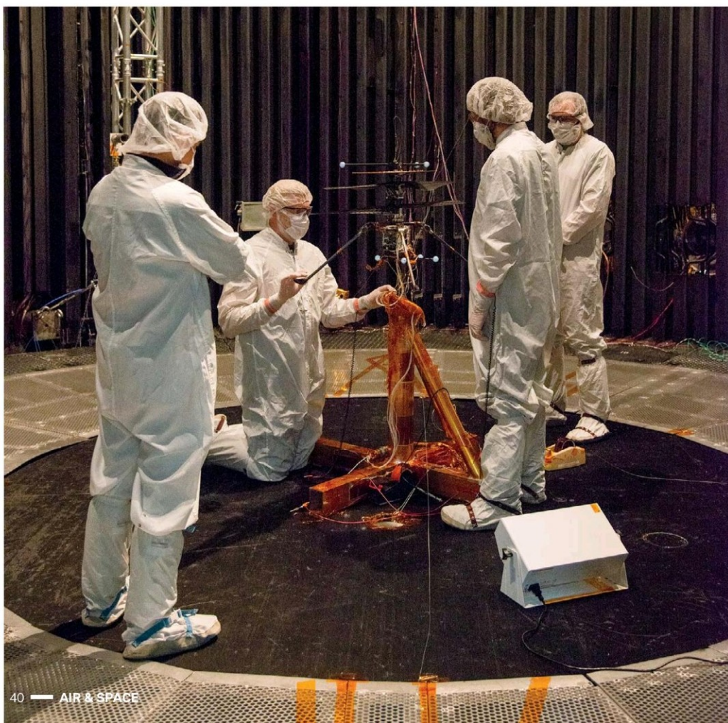
← On January 17, 2018, members of the Mars Helicopter team prepare the vehicle for a crucial test in JPL’s historic 25-foot vacuum chamber. The fully autonomous risk-reduction flight went off without a hitch.
