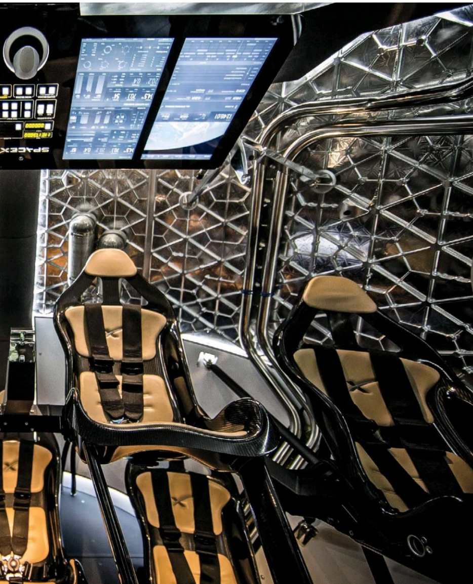
The no-cockpit interior of the Crew Dragon shows how automation will change spaceflight. ISS commuters can steer if needed, but will often be along for the ride.
