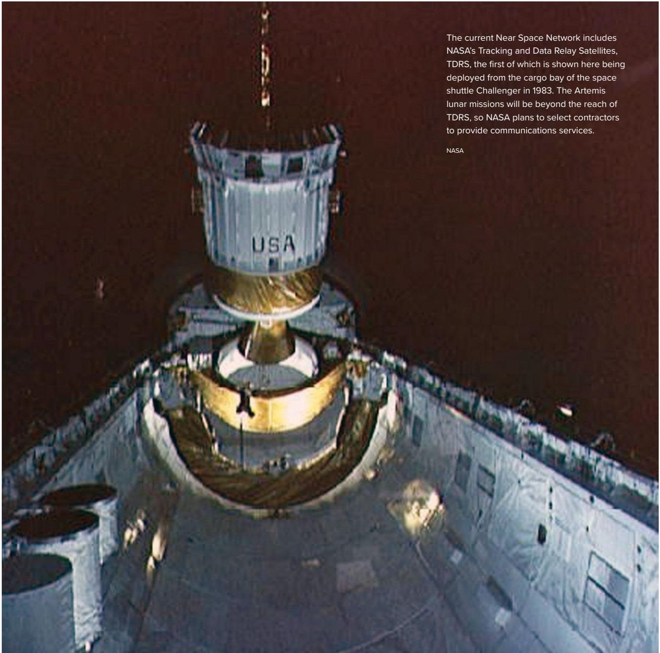
The current Near Space Network includes NASA's Tracking and Data Relay Satellites, TDRS, the first of which is shown here being deployed from the cargo bay of the space shuttle Challenger in 1983. The Artemis lunar missions will be beyond the reach of TDRS, so NASA plans to select contractors to provide communications services.
