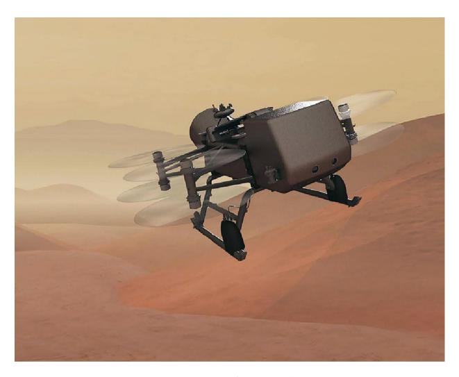
▲ Titan's atmosphere is believed to be four times denser than Earth's, which should make it easier for an aircraft to generate lift. Dragonfly mission architects have taken advantage of that fact in designing an octocopter that would make short flights on Titan.
