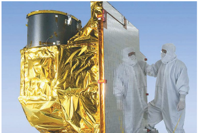
▲ NOAA planned to use the same Advanced Baseline Imager design on all four satellites in the GOES-R series, but a clogged cooling system on the GOES-17 camera prompted a redesign. NOAA
