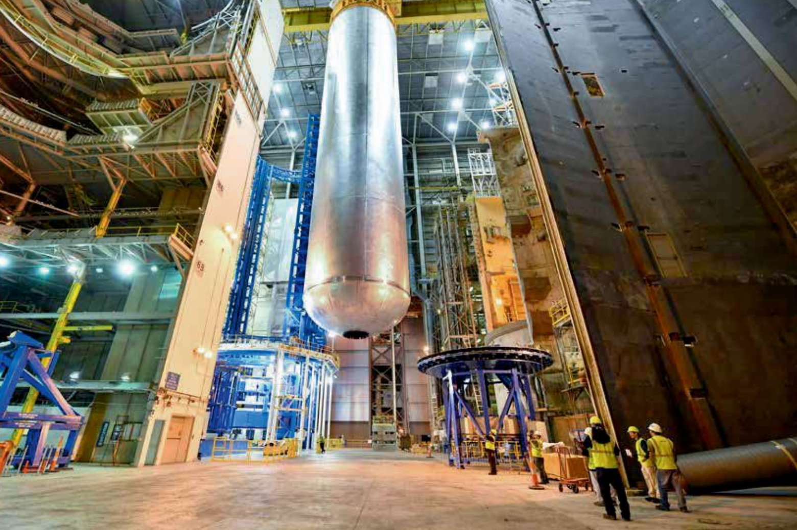
▲ The liquid hydrogen tank for the core stage of the first Space Launch System after welding was finished at NASA's Michoud Assembly Facility in Louisiana.
