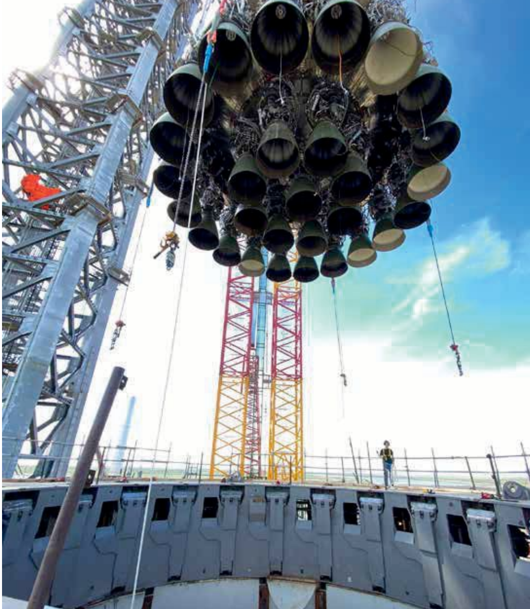
◀ A Super Heavy booster is moved by crane to the launch pad at SpaceX's Starbase facility in Texas. Each of the company's Starship launch vehicles will have a single Super Heavy booster as its core. The one in the photo has 29 Raptor engines, but Elon Musk has said operational versions could be powered by 33.
