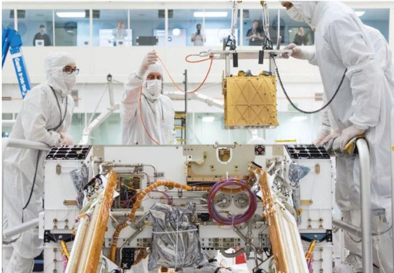
The **Mars Oxygen In-Situ Resource Utilization Experiment**, or **MOXIE**, the first ISRU project to be launched to another planet, began its journey to Mars aboard the Perseverance rover in July. MOXIE will demonstrate solid oxide electrolysis processing of the thin carbon dioxide atmosphere to produce 6-10 grams of oxygen each hourlong opportunity over the course of the Martian year.
